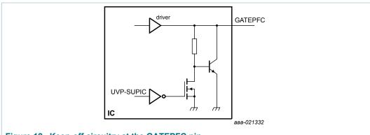
Figure 12. Keep-off circuitry at the GATEPFC pin
