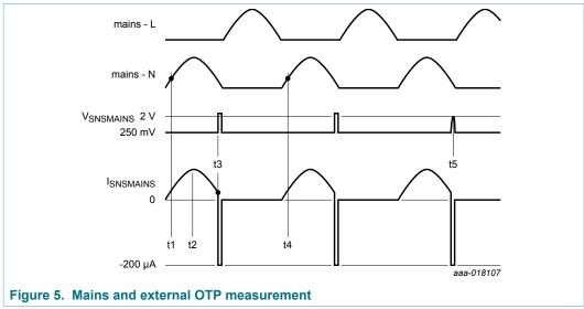
At t1. the voltage at the SNSMAINS pin is internally regulated to V<sub>read(SNSMAINS)</sub> (250 mV). The current into the SNSMAINS pin is a measure of the system input mains voltage. The TEA19162T continuously measures the SNSMAINS current and waits until it detects a peak in the measured current (t2). This peak current value is internally stored and used as an input for the brownout/brownin detection and the mains compensation.
