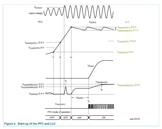
The exact start-up sequence of the PFC depends on the availability of start-up conditions (brownin level,  $V_{start(SUPIC)}$  of the PFC, and  $I_{en(PFC)}$ ).
