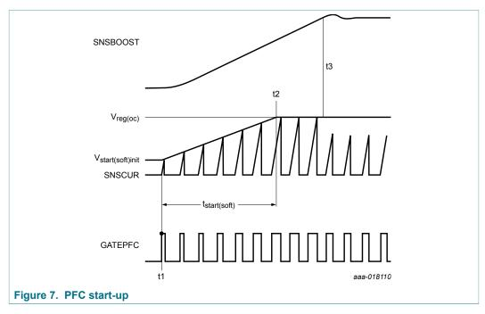
At t1, all conditions to start up the PFC are fulfilled. The maximum voltage on the SNSCUR pin is limited to  $V_{start(soft)init}$  (125 mV). When the PFC starts switching, the maximum SNSCUR voltage is increased to  $V_{reg(oc)}$  within a time period of  $t_{start(soft)}$  (3.62 ms) or until the  $t_{on}$  regulation limits the on-time of the PFC external MOSFET.
