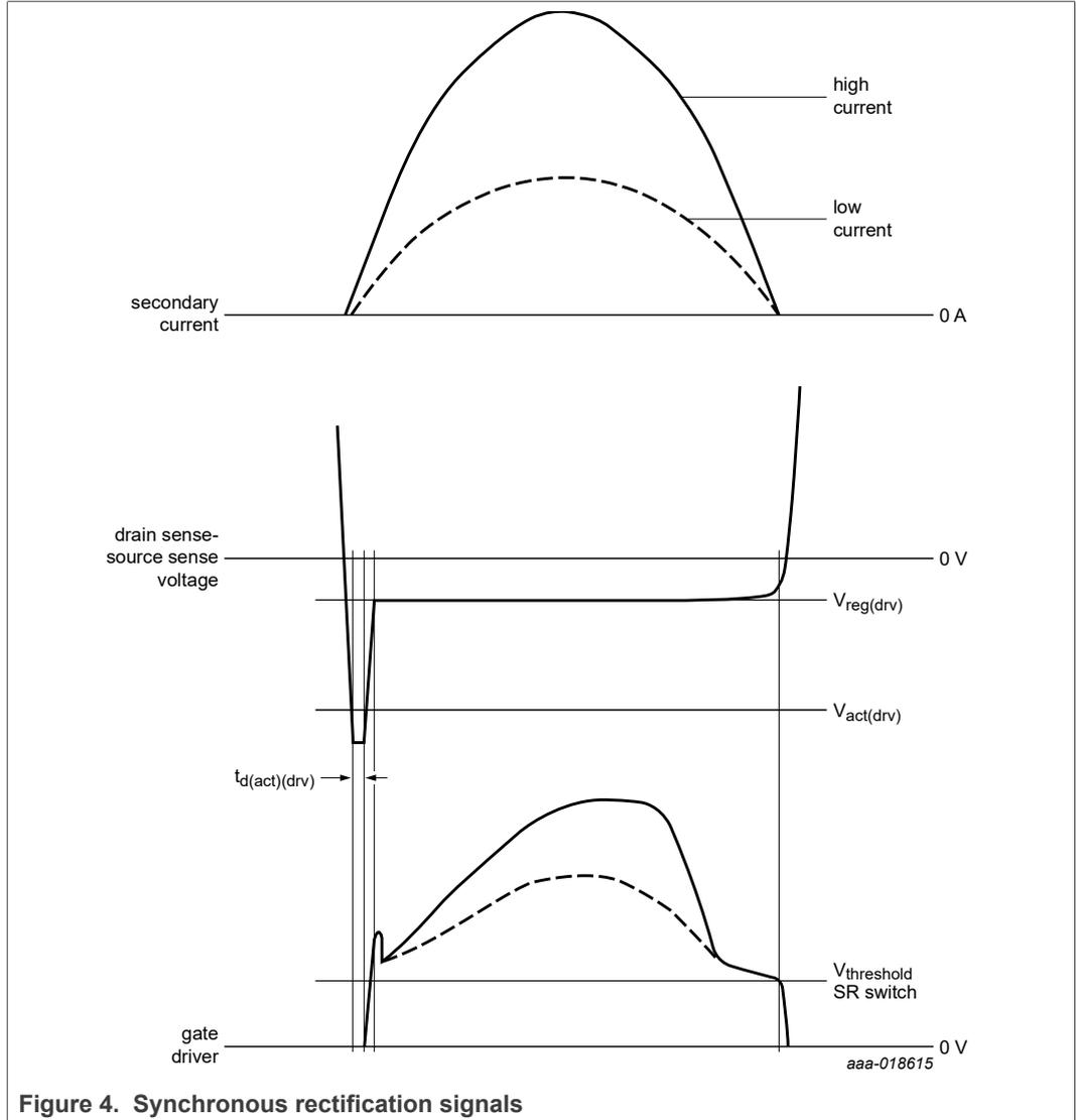
Figure 4. Synchronous rectification signals
