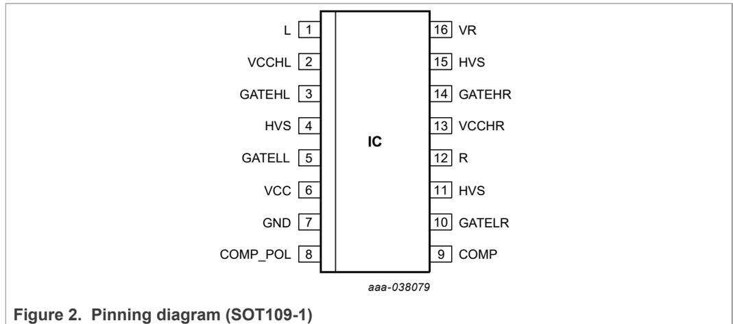
Figure 2. Pinning diagram (SOT109-1)
