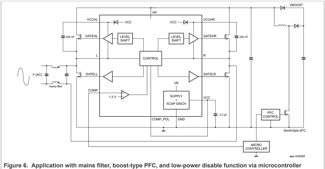
Figure 6. Application with mains filter, boost-type PFC, and low-power disable function via microcontroller
