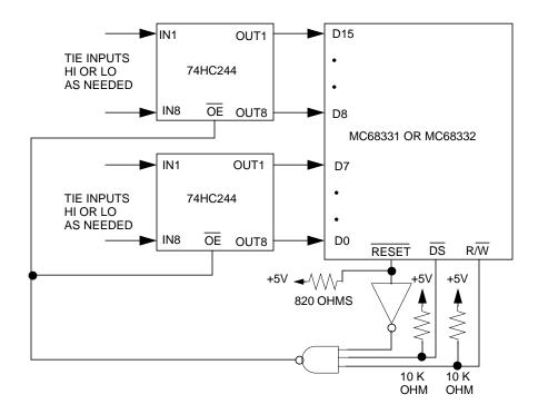
NOTE: THIS CIRCUIT PROTECTS MEMORY ACCESSES THAT ARE CURRENTLY IN PROGRESS. THAT IS, IF THE RESET PIN IS ASSERTED DURING AN EXTERNAL MEMORY ACCESS, THE OUTPUTS OF THE 74HC244'S CANNOT BE TURNED ON UNTIL THE EXTERNAL MEMORY IS COMPLETED, THUS PREVENTING THE CORRUPTION OF DATA BEING WRITTEN TO THE EXTERNAL MEMORY DEVICE. IF THIS IS NOT A CONCERN TO THE SYSTEM, THEN THE RESET PIN CAN SIMPLY BE TIED DIRECTLY TO THE OE PINS OF THE 74HC244.
