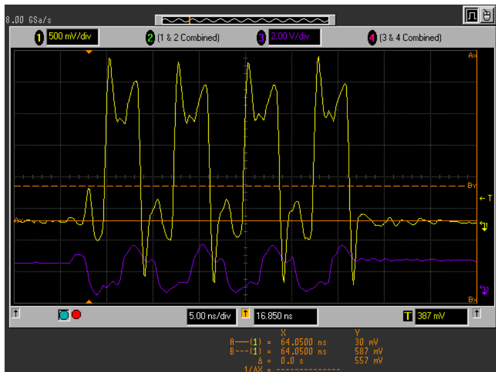
Figure 9. Scope Capture of DQS0 with DDR2 Drive Strength
