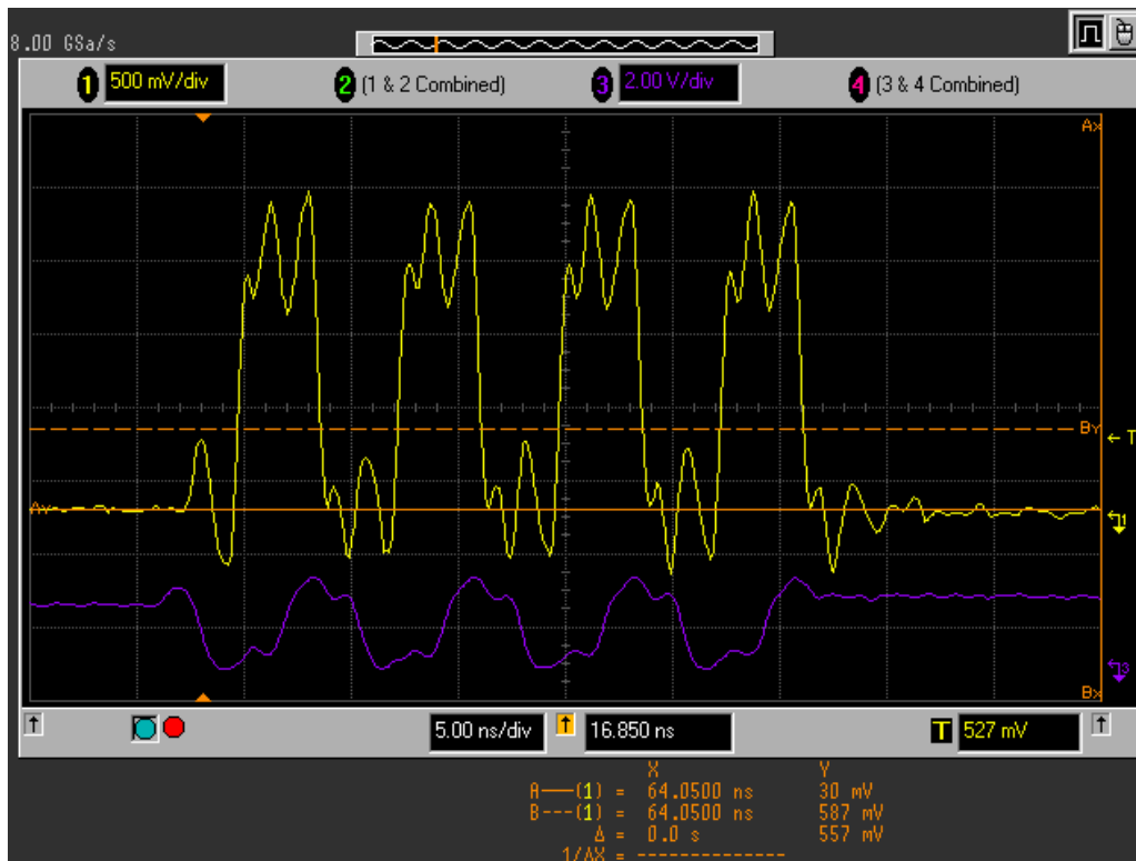
Figure 5. Scope Capture of Filtered DQS0 Signal
