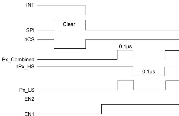
The horizontal divisions are not to scale, they are a reference to show the sequence of operation. Either individual nPx\_HS and Px\_LS or nPx\_Combined may be used. nPx\_Combined is defined as both nPx\_HS and Px\_LS tied together or operated to the same logic level simultaneously.
