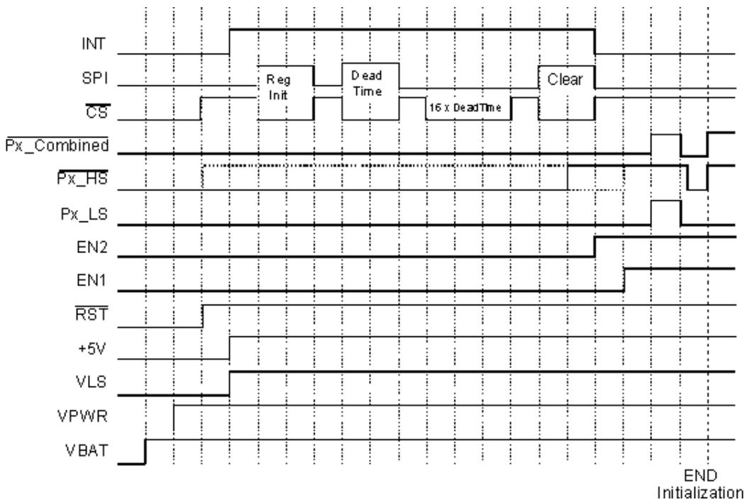
The horizontal divisions are not to scale, they are a reference to show the sequence of operation. Either individual nP<sub>x</sub>\_HS and P<sub>x</sub>\_LS or nP<sub>x</sub>\_Combined may be used. nP<sub>x</sub>\_Combined is defined as both nP<sub>x</sub>\_HS and P<sub>x</sub>\_LS tied together or operated to the same logic level simultaneously.
