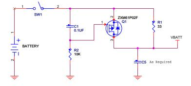
Figure 2. Soft-start Circuit for Battery Operation
