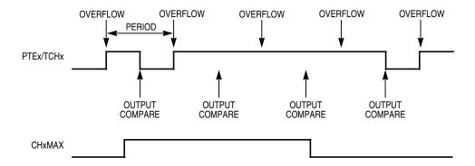
**NOTE:** The PWM 0% duty cycle is defined as output low all of the time. To generate the 0% duty cycle, select clear output on compare and then clear the TOVx bit (CHxMAX=0).
