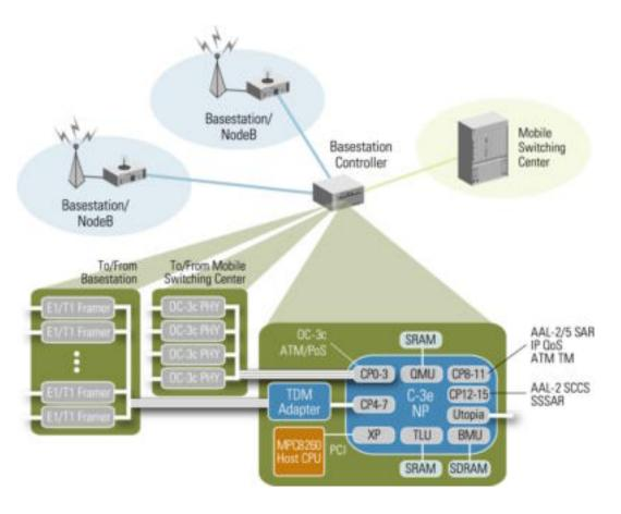
Further, as protocols evolve, the NPs can be reprogrammed in software to address new requirements.
