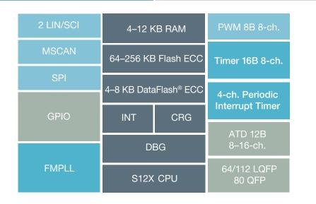
The S12XS family features a streamlined set of on-chip peripheral, memory and package options optimized for automotive body and passenger comfort applications. Compact packaging makes these devices suitable for space-constrained applications, such as small actuators, sensor modules and columnintegrated modules.
