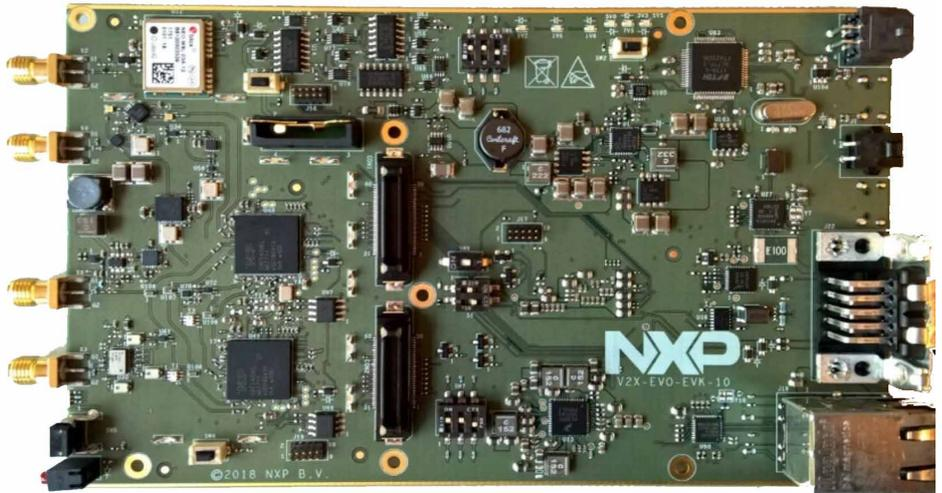
The EVK is designed to fit small form factors to also allow for seamless integration into cars and roadside units.
