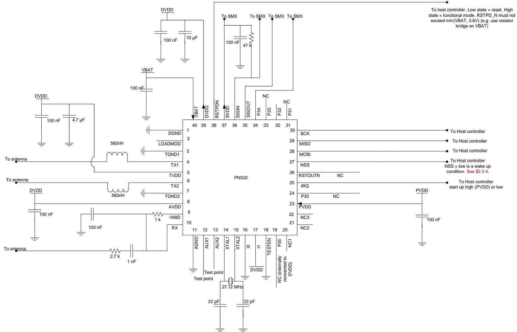
Fig 2. SPI PN532C106 application diagram
