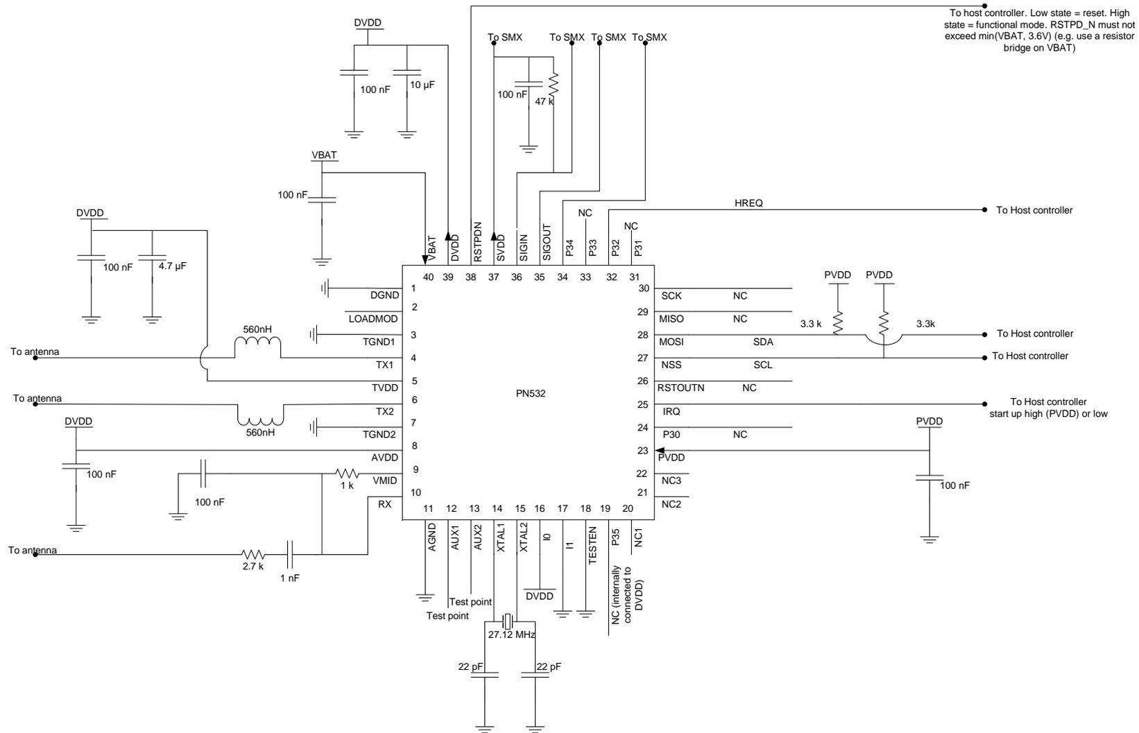
Fig 1. I2C PN532C106 application diagram
