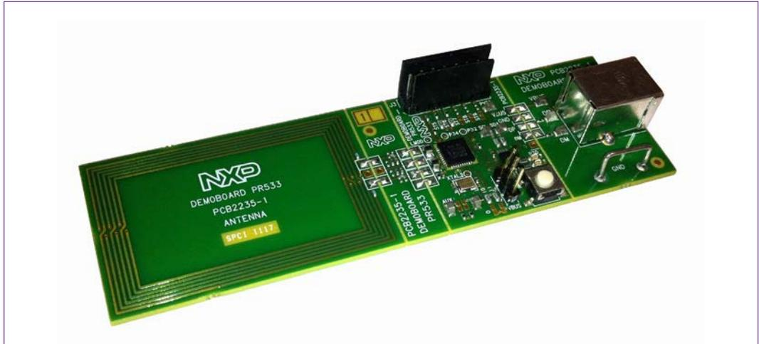
Fig 1. PR533 Evaluation board
