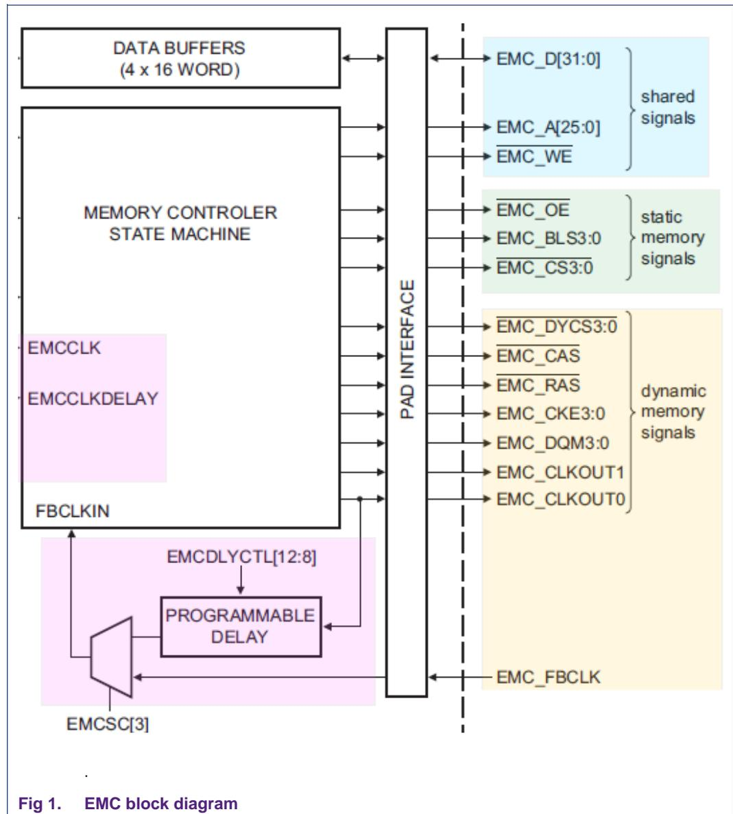
Fig 1. EMC block diagram
