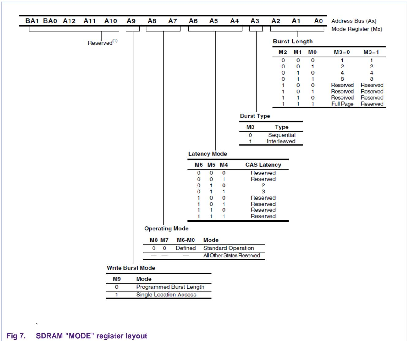
Fig 7. SDRAM "MODE" register layout
