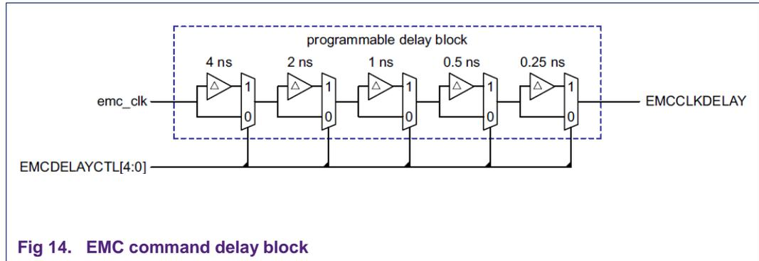
Fig 14. EMC command delay block
