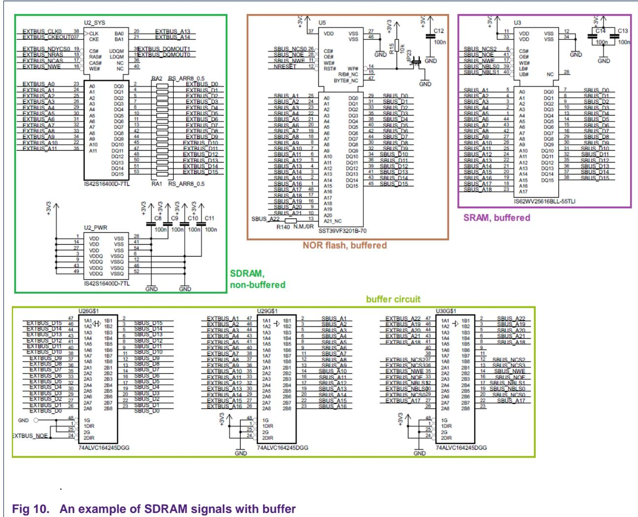
Fig 10. An example of SDRAM signals with buffer
