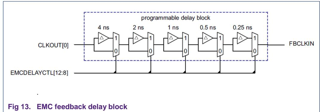
**Fig 13. EMC feedback delay block**
