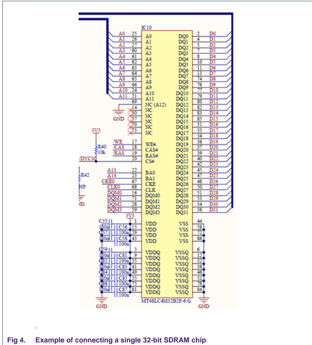
Fig 4. Example of connecting a single 32-bit SDRAM chip
