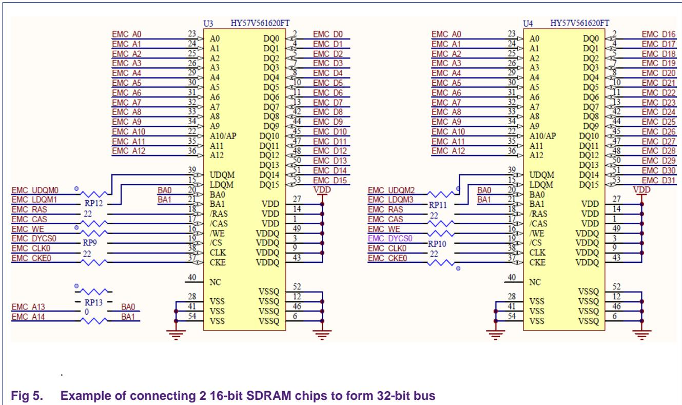
Fig 5. Example of connecting 2 16-bit SDRAM chips to form 32-bit bus
