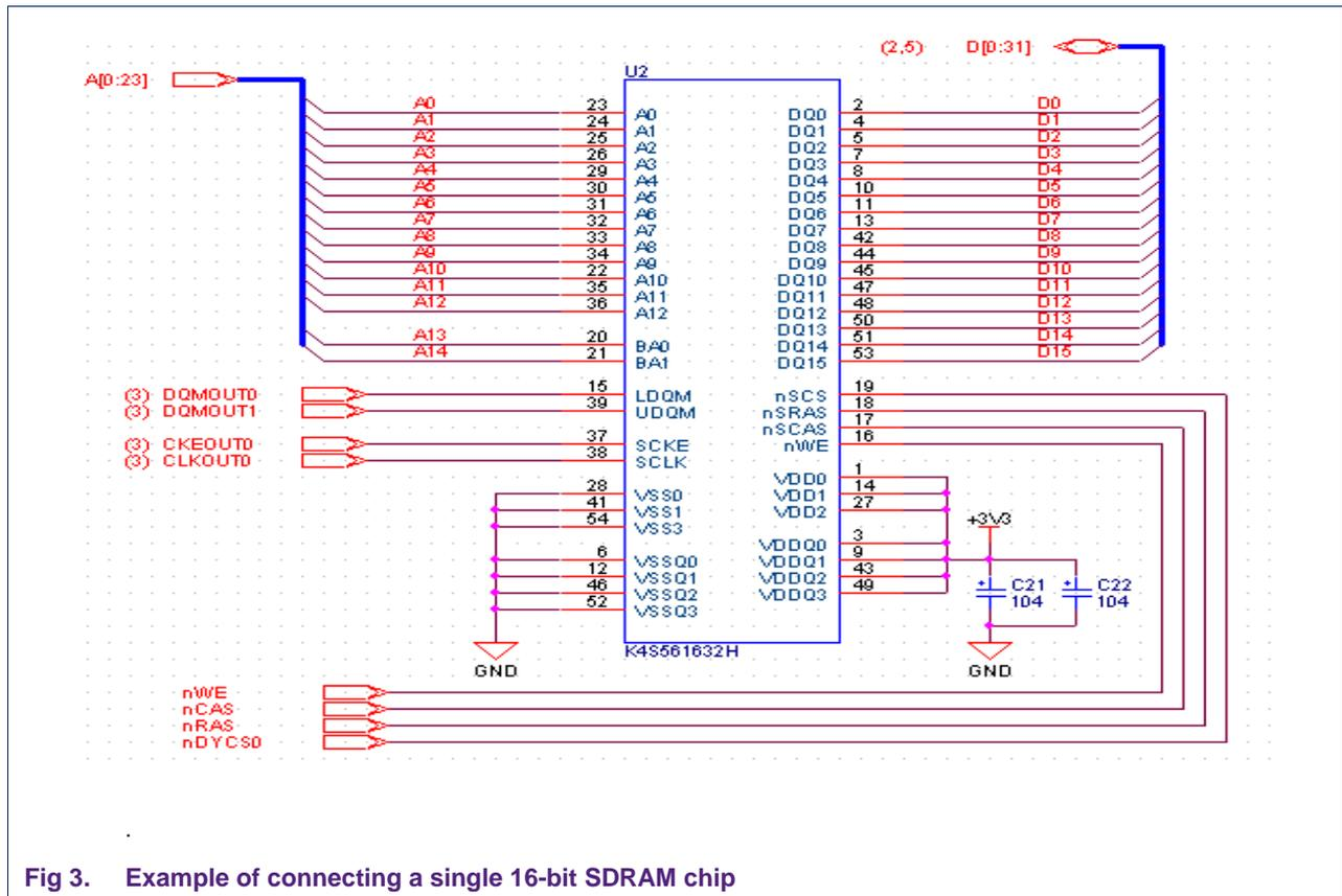
Fig 3. Example of connecting a single 16-bit SDRAM chip
