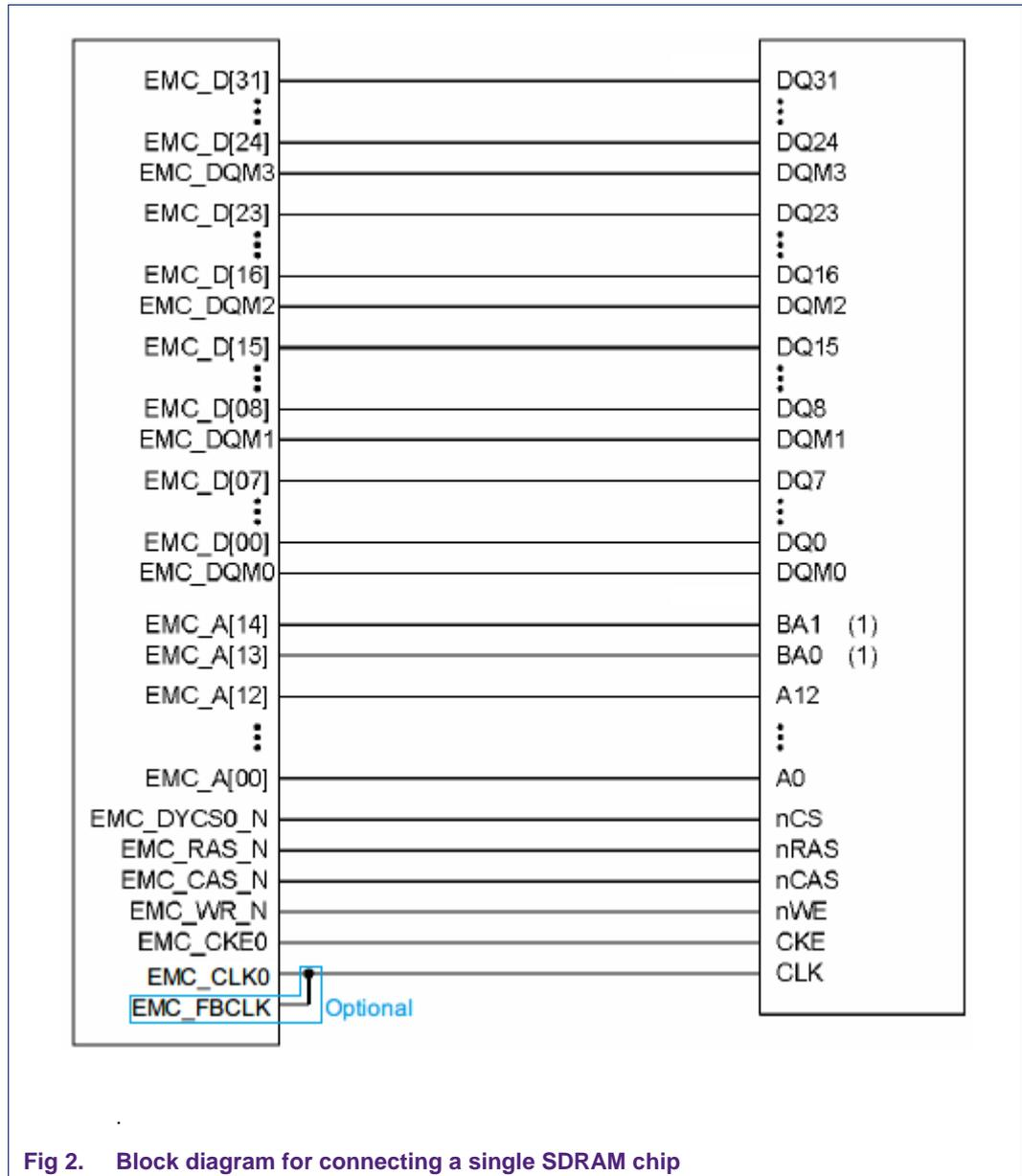
Fig 2. Block diagram for connecting a single SDRAM chip
