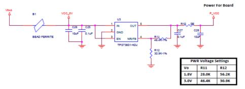
Fig 4. QN9080 USB dongle board power supply
