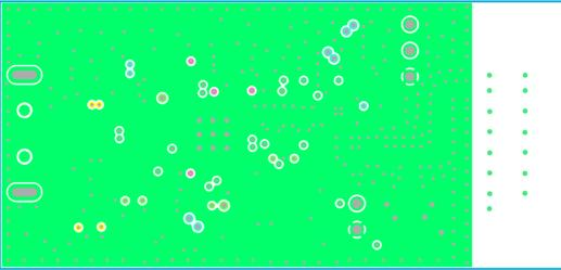
Fig 9. Range extender solution with SKY66114 GND layer
