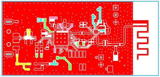
Fig 7. Range extender solution with SKY66114 top etch layer
