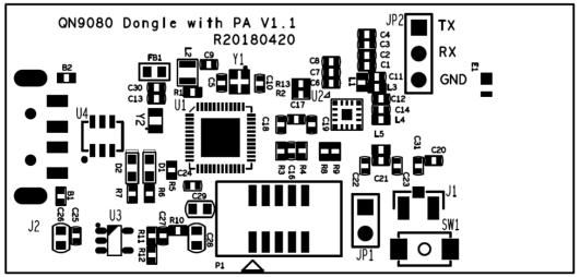
Fig 8. Range extender solution with SKY66114 top silkscreen layer
