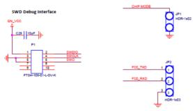
Fig 6. QN9080 USB dongle board debug interface
