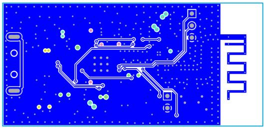
Fig 11. Range extender solution with SKY66114 bottom layer
