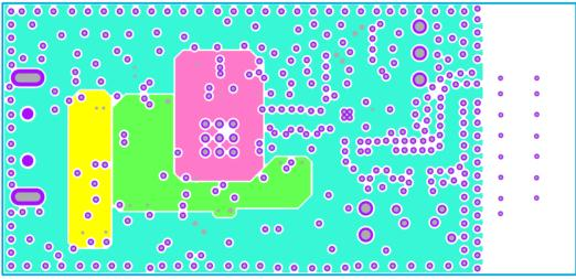
Fig 10. Range extender solution with SKY66114 PWR layer
