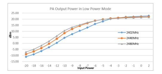
Fig 14. PA output power in low-power mode
