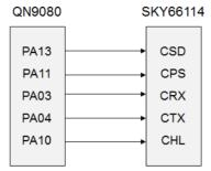
Fig 2. QN9080 logic control pins
