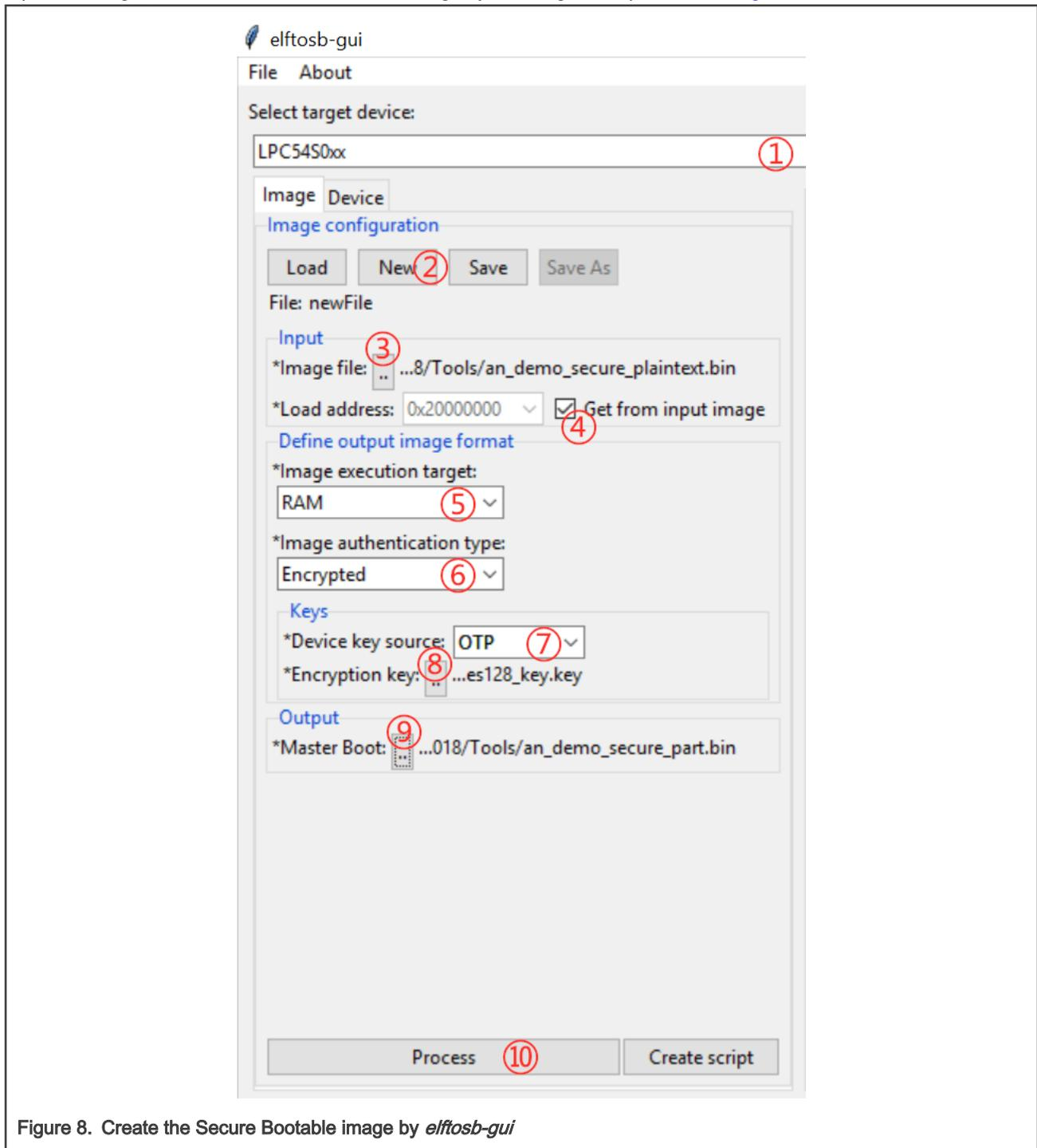
Figure 8. Create the Secure Bootable image by *elftosb-gui*
