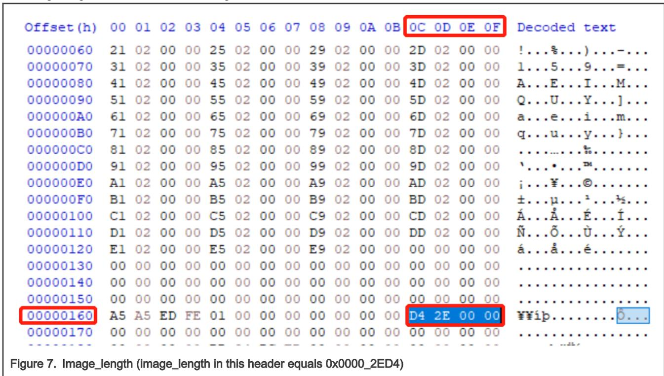
Figure 7. Image\_length (image\_length in this header equals 0x0000\_2ED4)
