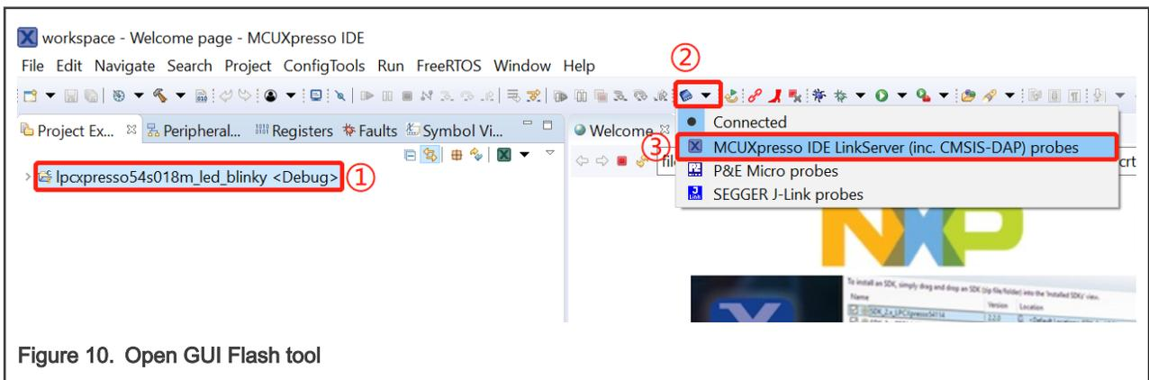
Figure 10. Open GUI Flash tool
