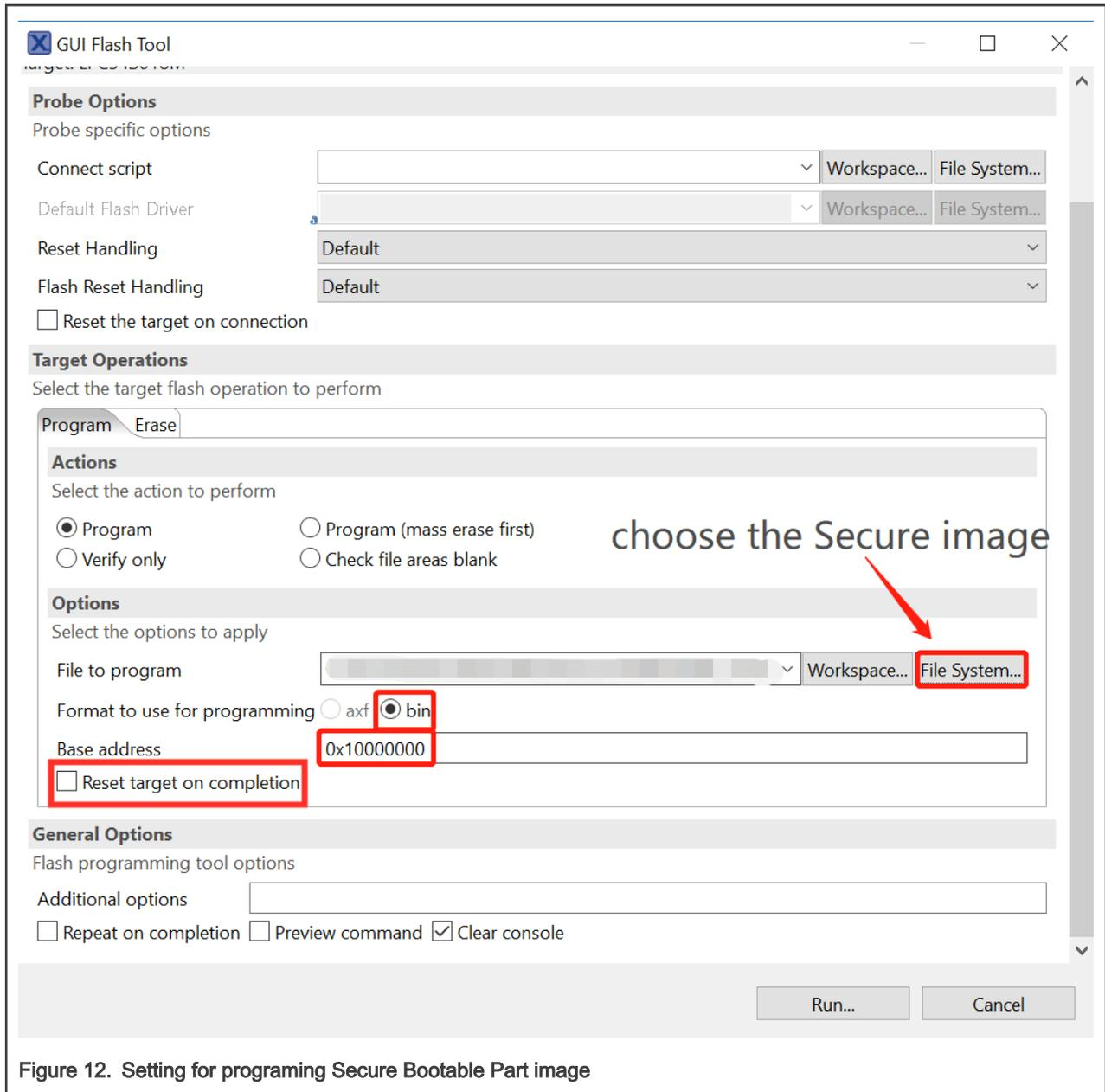
Figure 12. Setting for programming Secure Bootable Part image
