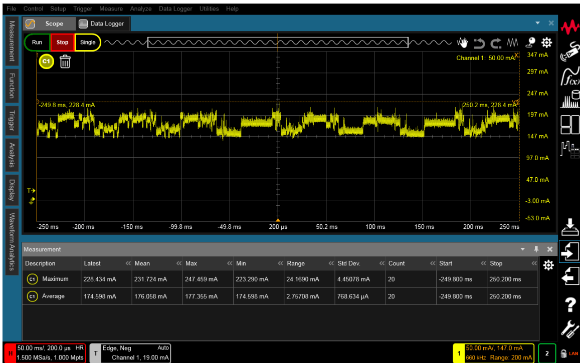
Figure 6. +5V Current consumption of SLN-VIZN-IOT kit – running userid_oobe .
