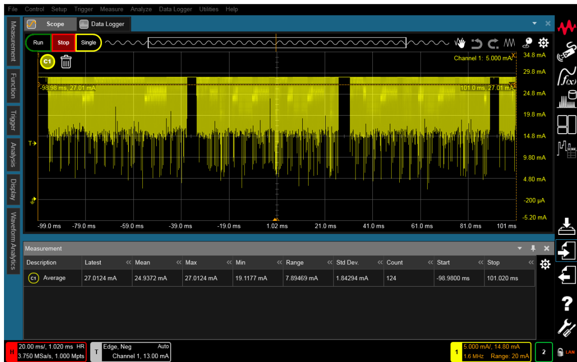
Figure 5. +3.3V Current consumption of SDRAM – Running userid_oobe
