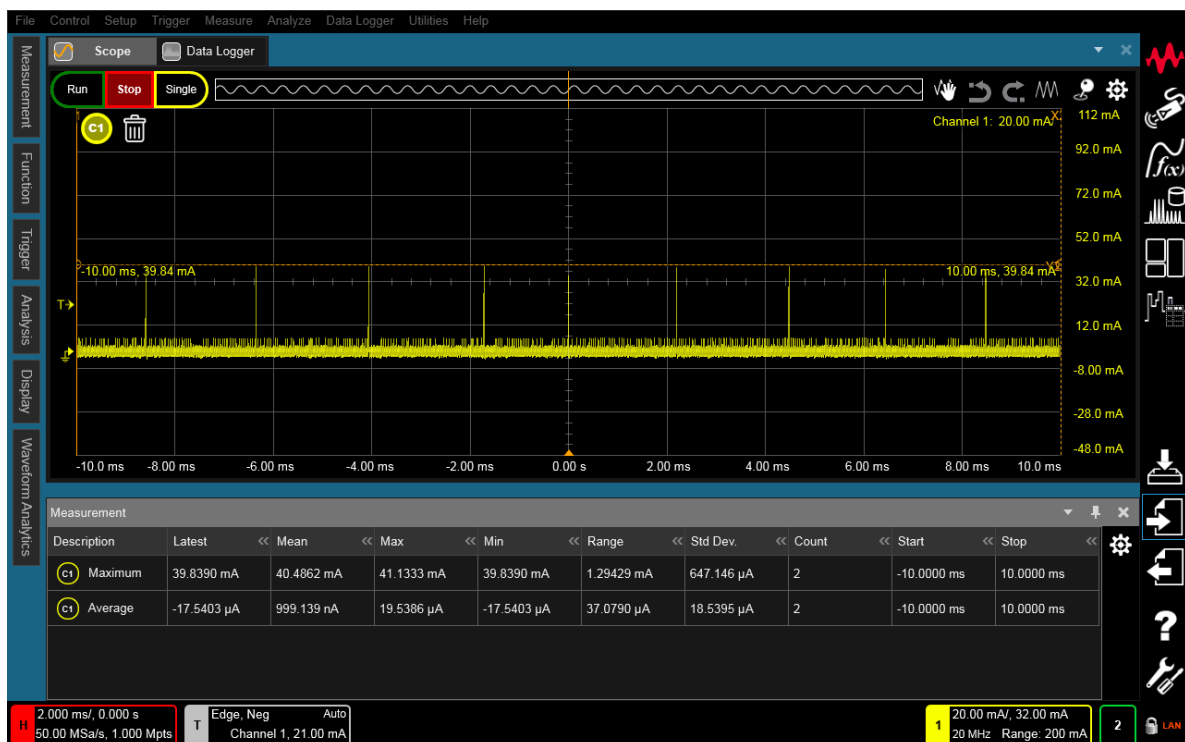
Figure 4. +3.3V Current consumption of i.MXRT106F – Suspend mode.
