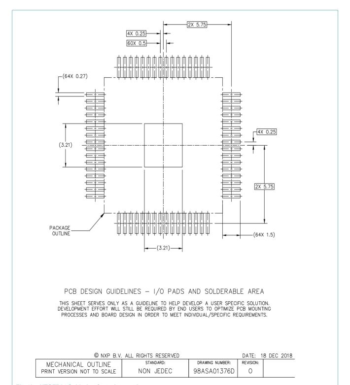
Fig 40. HTQFP64 Soldering footprint part 2
