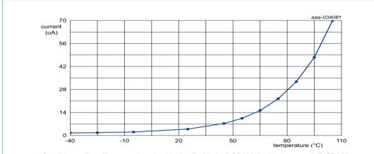
Conditions: all oscillators and analog blocks disabled; all SRAM disabled except 4KB SRAM powered. Flash powered down.
