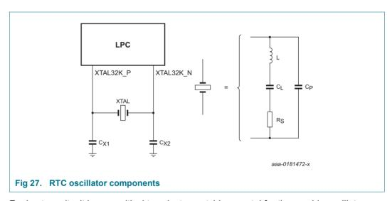
For best results, it is very critical to select a matching crystal for the on-chip oscillator. Load capacitance (CL), series resistance (RS), and drive level (DL) are important parameters to consider while choosing the crystal.
