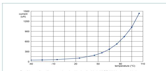
Conditions: all oscillators and analog blocks disabled. All SRAM blocks enabled.
