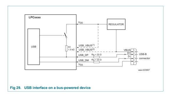
Two options exist for connecting VBUS to the USB\_VBUS pin:
