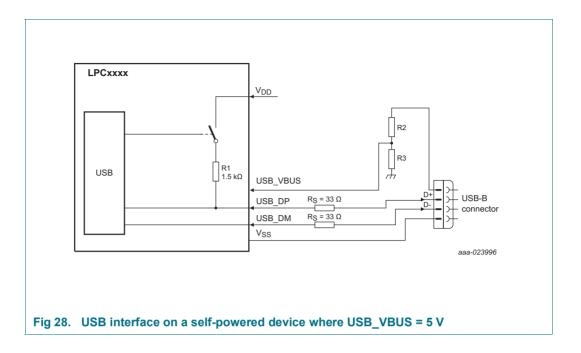
The internal pull-up (1.5 kW) can be enabled by setting the DCON bit in the DEVCMDSTAT register to prevent the USB from timing out when there is a significant delay between power-up and handling USB traffic. External circuitry is not required.
