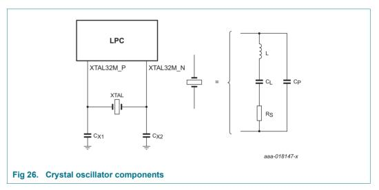
For best results, it is very critical to select a matching crystal for the on-chip oscillator. Load capacitance (CL), series resistance (RS), and drive level (DL) are important parameters to consider while choosing the crystal.
