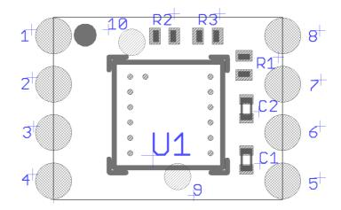
The PCB measures 4.8x6.0mm (length x width). The total height of the board assembly is 1.45mm±0.3. The castellated holes have a pitch of 1.27mm. The NxH5104\_SOIC\_ADB replaces an 8-SOIC JEDEC compliant device.
