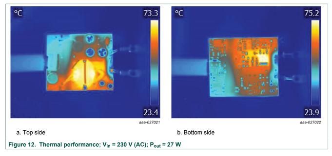
**Note:** Typical temperature distribution at  $T_{amb}$  = 25 °C; PCB in free air, natural convection, and radiation only.
