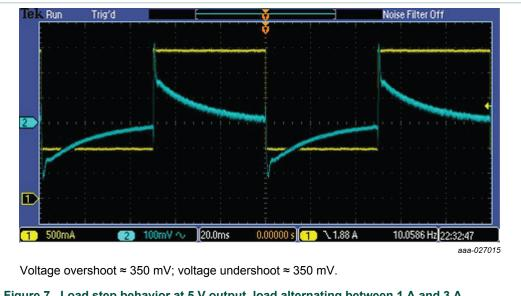
Figure 7. Load step behavior at 5 V output, load alternating between 1 A and 3 A
