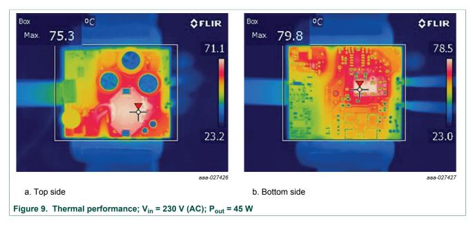
**Note:** Typical temperature distribution at  $T_{amb}$  = 25 °C; PCB in free air, natural convection, and radiation only. For the TEA1936xDB1521 demo board, the voltage levels must not exceed 20 V also. Current limit levels must not exceed 3 A. Power limit levels must not exceed 45 W.
