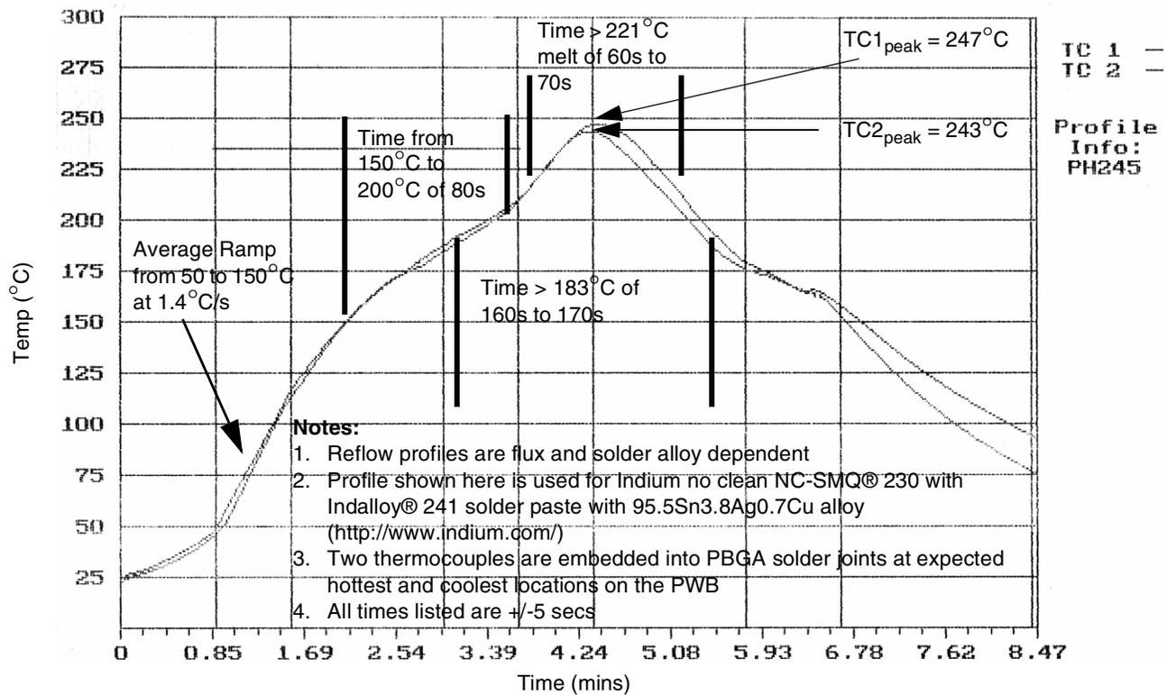
Figure 4. Typical Freescale Pb-Free Board Assembly Reflow Profile
