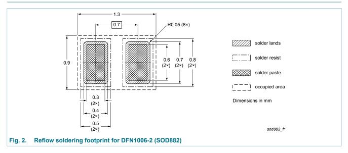
plastic, leadless ultra small package; 2 terminals; 0,65 mm pitch; 1 mm x 0.6 mm x 0.48 mm body
