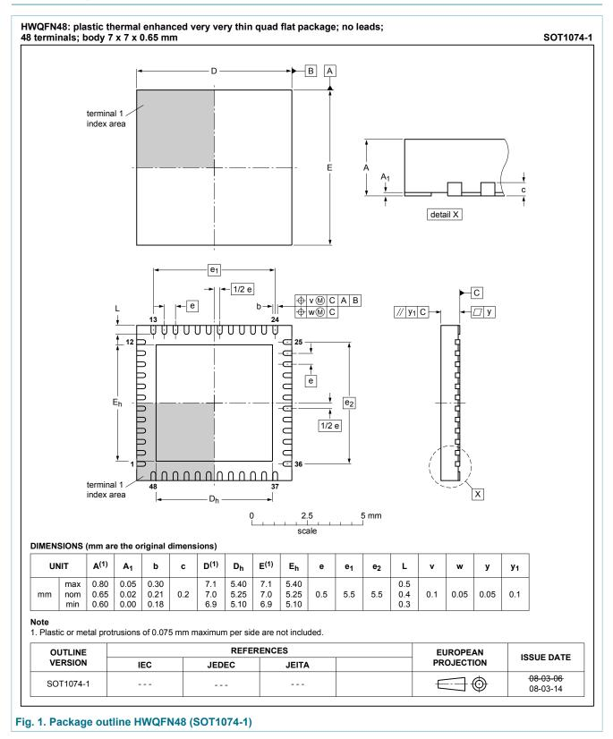
plastic thermal enhanced very very thin quad flat package; no leads; 48 terminals; body 7 x 7 x 0.65 mm
