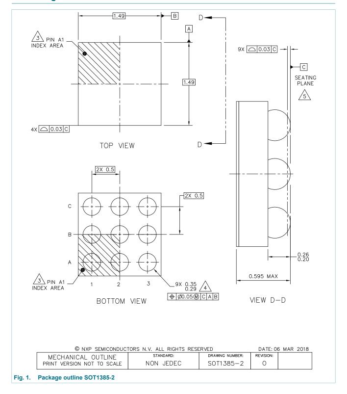
WLCSP9, wafer level chip-scale package; 9 bumps; 0.5 mm pitch, 1.49 mm x 1.49 mm x 0.555 mm body (backside coating included)
