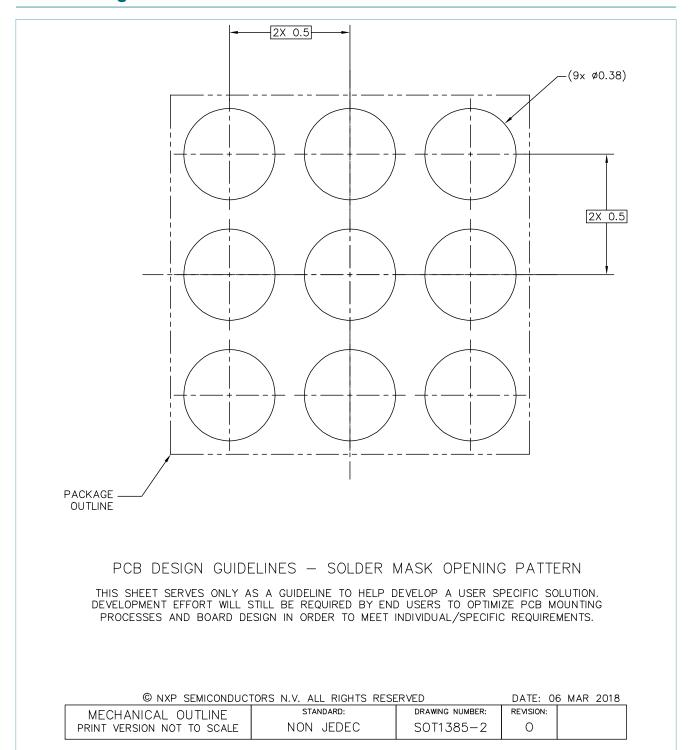
Fig. 3. Reflow soldering footprint for SOT1385-2
