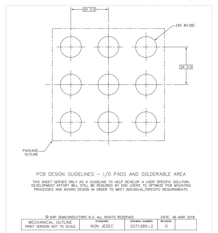
Fig. 4. Reflow soldering footprint part2 for WLCSP9 (SOT1385-2)
