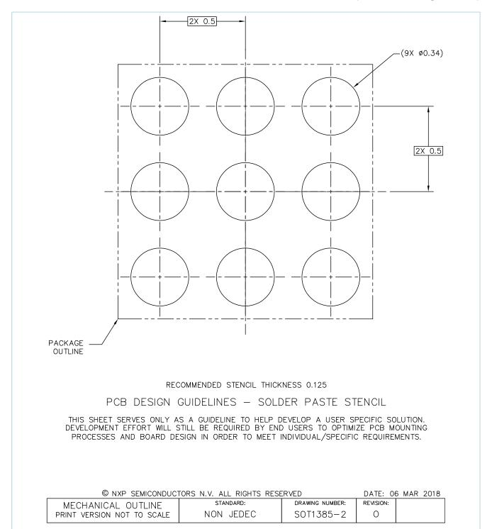
Fig. 5. Reflow soldering footprint part3 for WLCSP9 (SOT1385-2)
