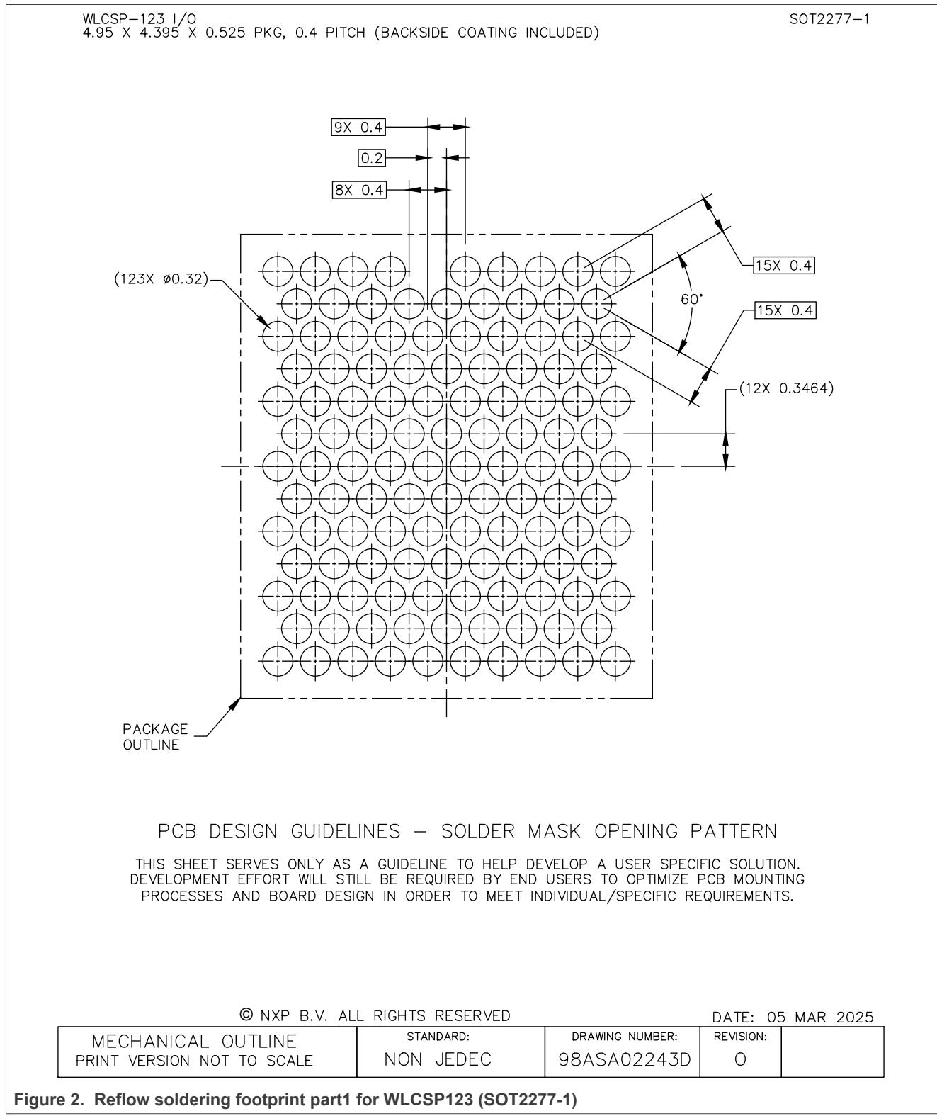
**WLCSP123, wafer level chip-size package, 123 terminals, 0.4 mm pitch, 4.95 mm x 4.395 mm x 0.525 mm body**
