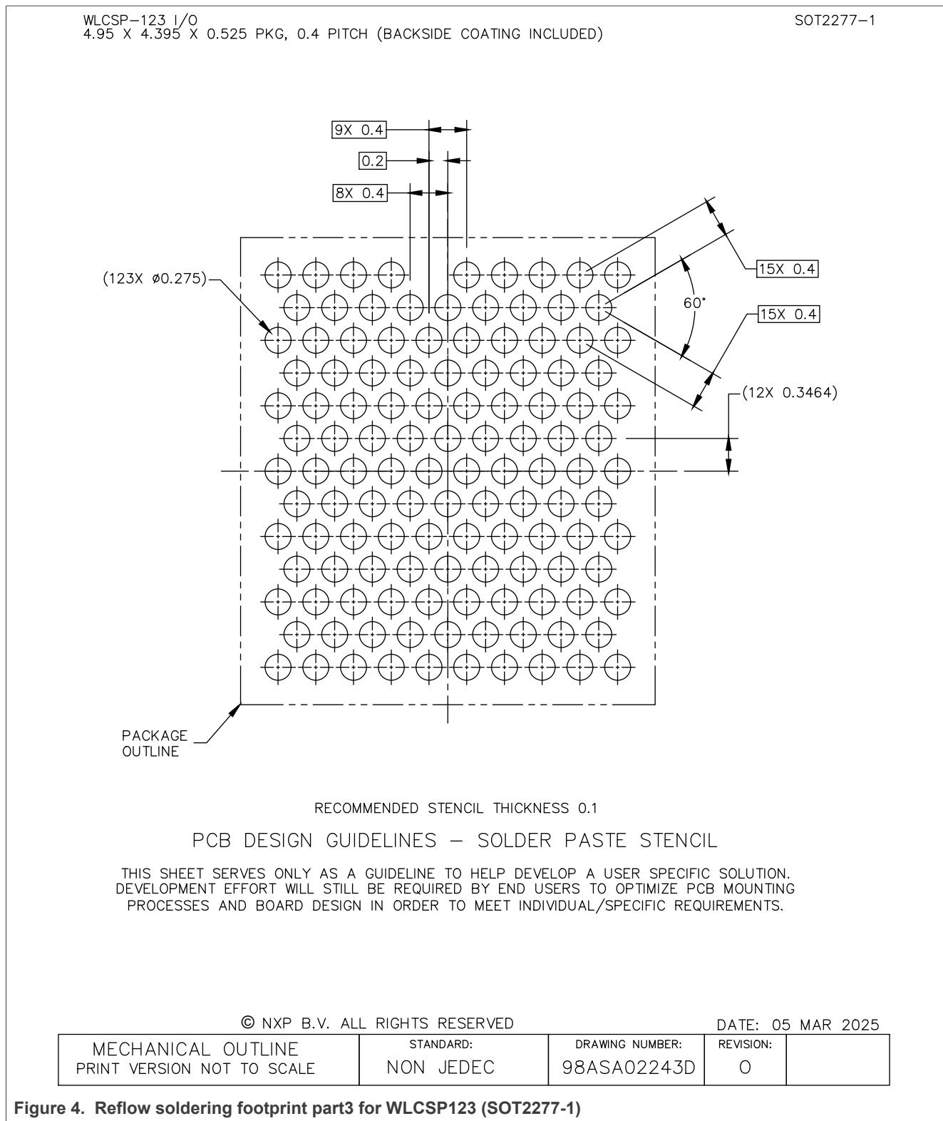
**WLCSP123, wafer level chip-size package, 123 terminals, 0.4 mm pitch, 4.95 mm x 4.395 mm x 0.525 mm body**WLCSP-123 I/O
