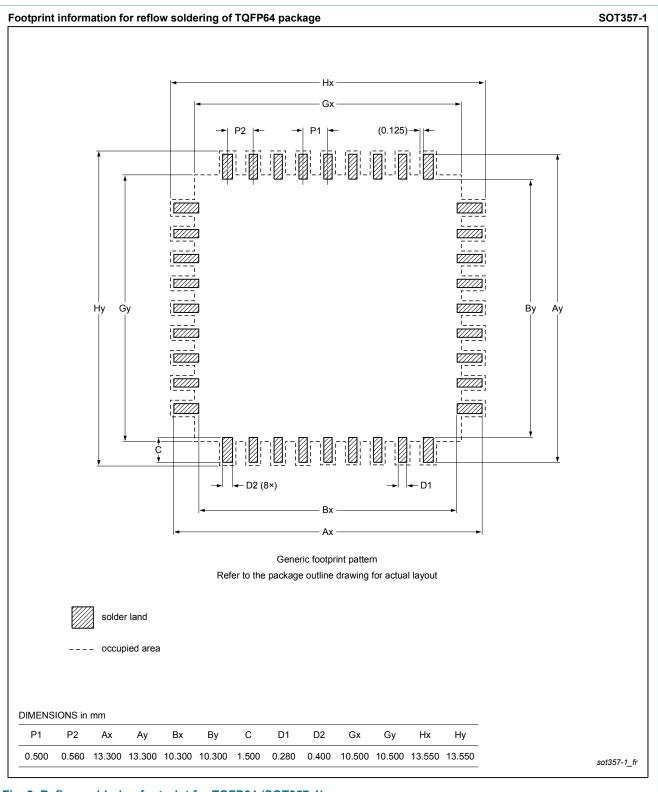
Fig. 2. Reflow soldering footprint for TQFP64 (SOT357-1)
