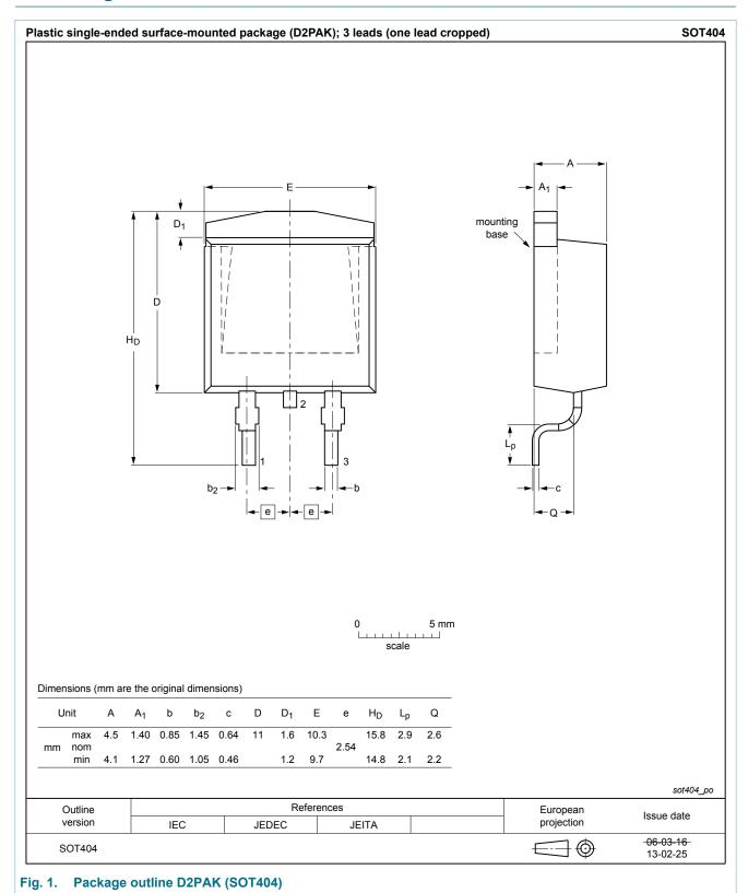
plastic single-ended surface-mounted package (D2PAK); 3 terminals (one lead cropped); 2.54 mm pitch; 11 mm x 10 mm x 4.3 mm body
