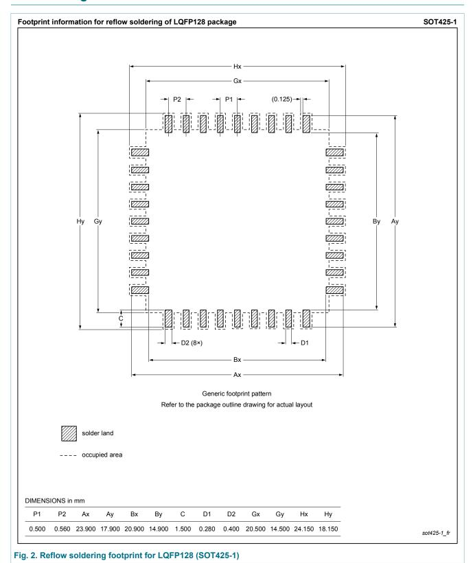
plastic low profile quad flat package; 128 leads; body 14 x 20 x 1.4 mm
