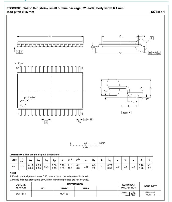
plastic thin shrink small outline package; 32 leads; body width 6.1 mm; lead pitch 0.65 mm
