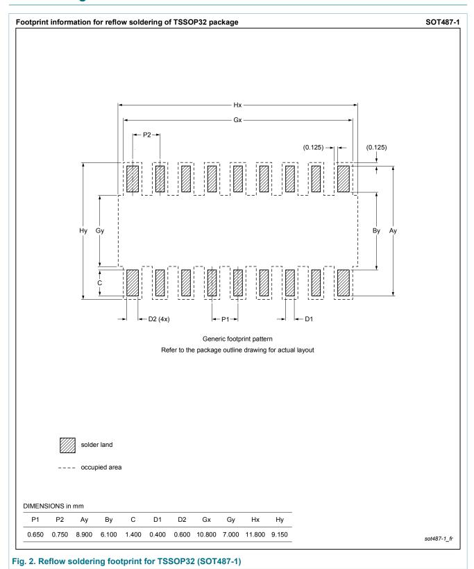
plastic thin shrink small outline package; 32 leads; body width 6.1 mm; lead pitch 0.65 mm
