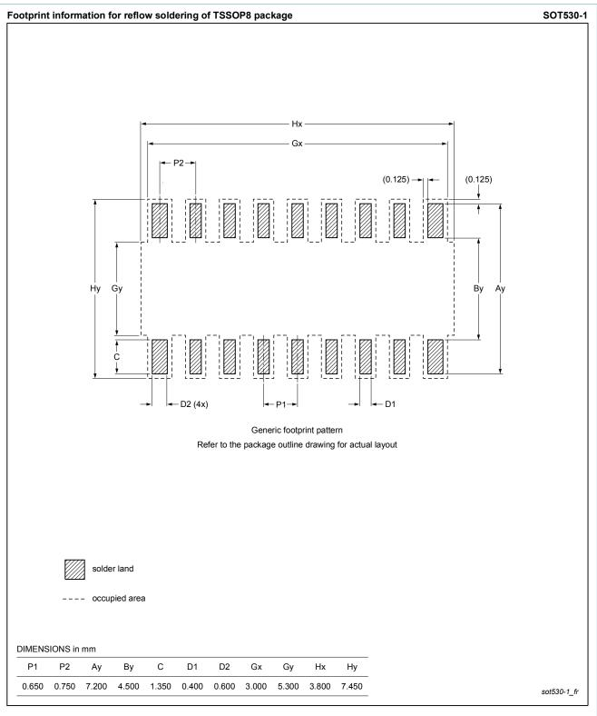
Fig. 2. Reflow soldering footprint for TSSOP8 (SOT530-1)
