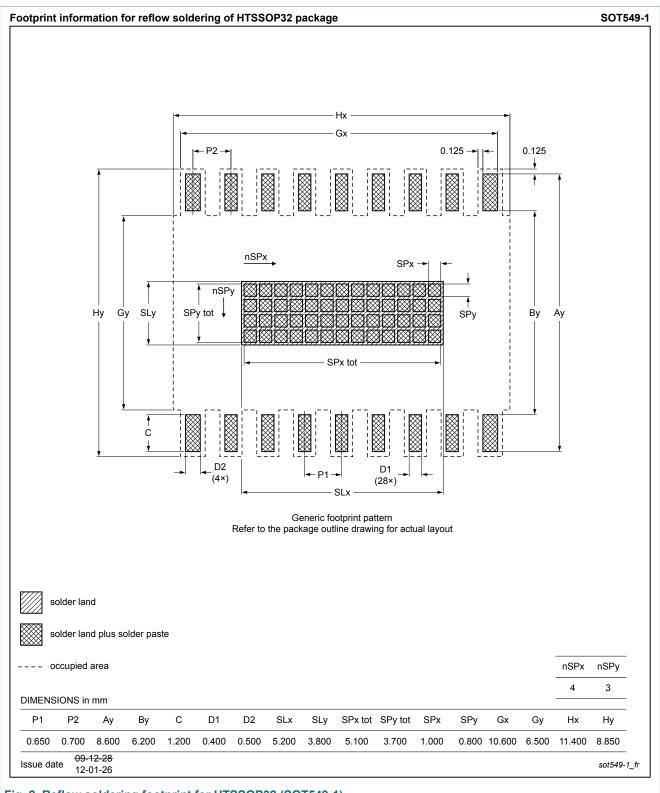
Fig. 2. Reflow soldering footprint for HTSSOP32 (SOT549-1)
