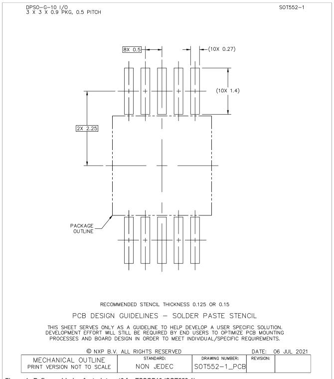
Figure 4. Reflow soldering footprint part3 for TSSOP10 (SOT552-1)
