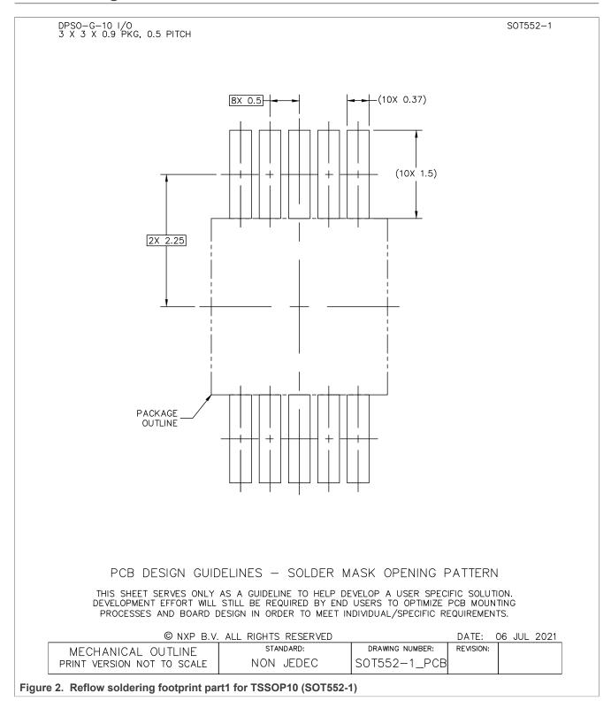
plastic, thin shrink small outline package; 10 leads; 0.5 mm pitch; 3 mm x 3 mm x 1.1 mm body
