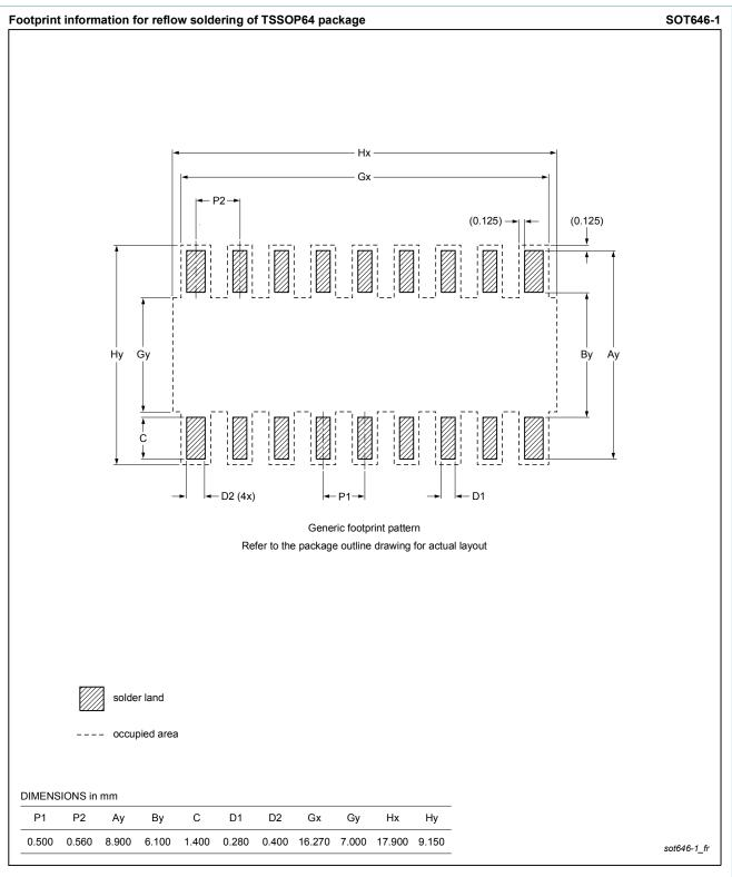
Fig. 2. Reflow soldering footprint for TSSOP64 (SOT646-1)
