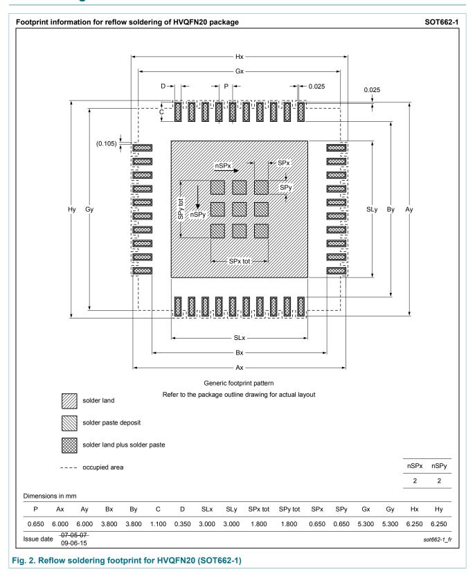
plastic thermal enhanced very thin quad flat package; no leads; 20 terminals; body 5 x 5 x 0.85 mm
