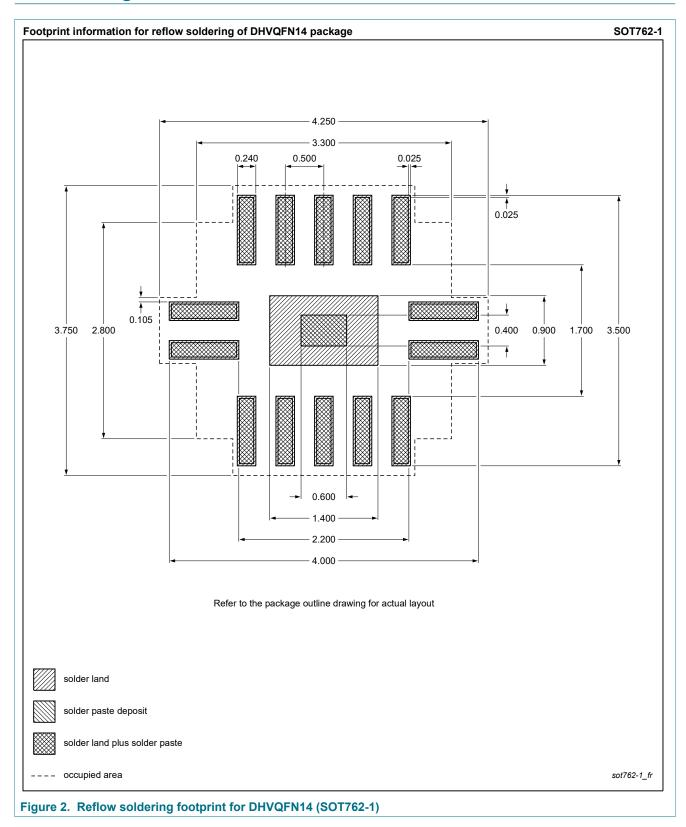
plastic, dual in-line compatible thermal enhanced very thin quad flat package; no leads; 14 terminals; 0.5 mm pitch; 2.5 mm x 3 mm x 0.85 mm body
