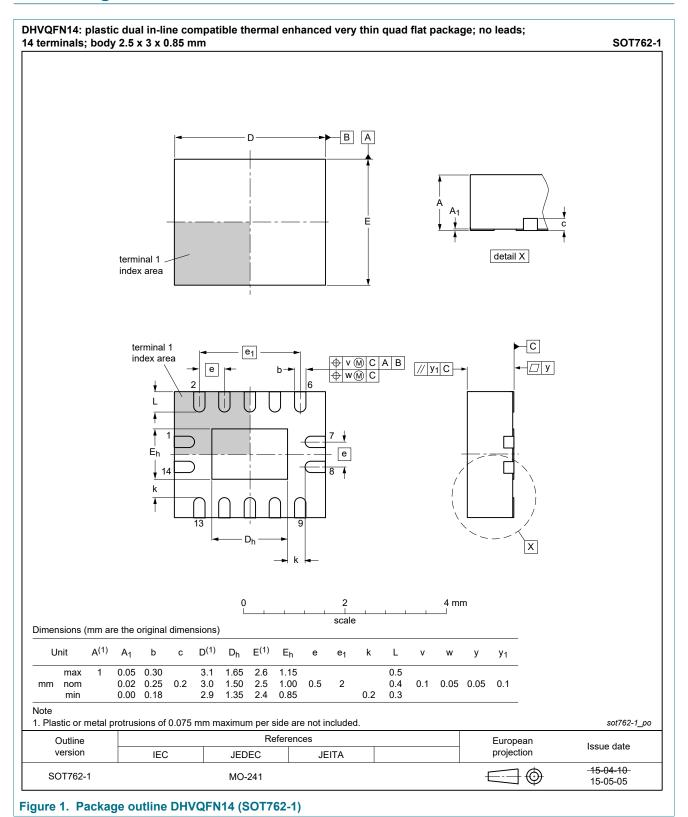
plastic, dual in-line compatible thermal enhanced very thin quad flat package; no leads; 14 terminals; 0.5 mm pitch; 2.5 mm x 3 mm x 0.85 mm body
