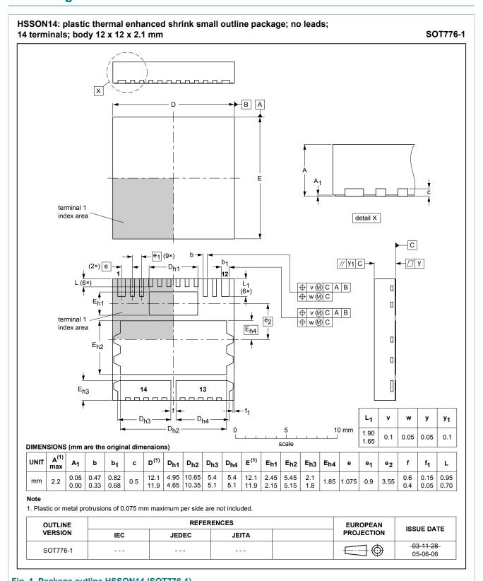
plastic thermal enhanced shrink small outline package; no leads; 14 terminals; body 12 x 12 x 2.1 mm
