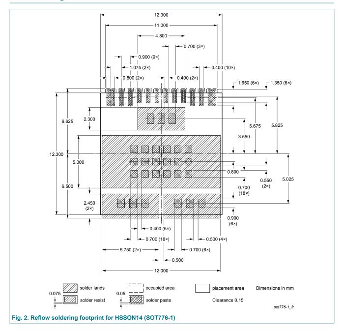
plastic thermal enhanced shrink small outline package; no leads; 14 terminals; body 12 x 12 x 2.1 mm
