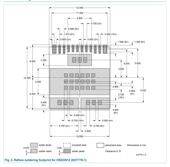
plastic thermal enhanced shrink small outline package; no leads; 14 terminals; body 12 x 12 x 2.1 mm
