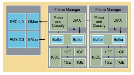
Figure 10. PowerQUICC Datapath Acceleration Architecture
