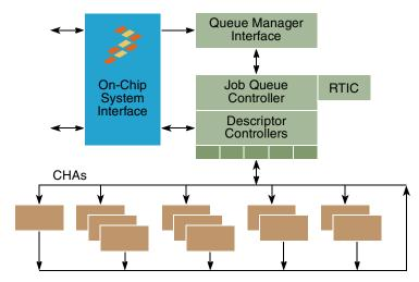
Figure 11. SEC 4.0 Block Diagram
