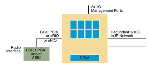
Figure 6. Wireless Infrastructure/Radio Node Controller
