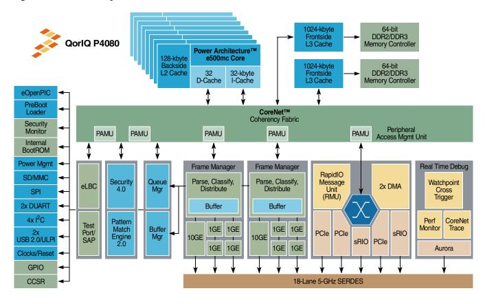
Figure 1. P4080 Preliminary Block Diagram
