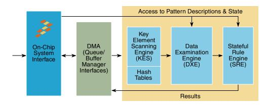
Figure 12. PME 2.0 Block Diagram
