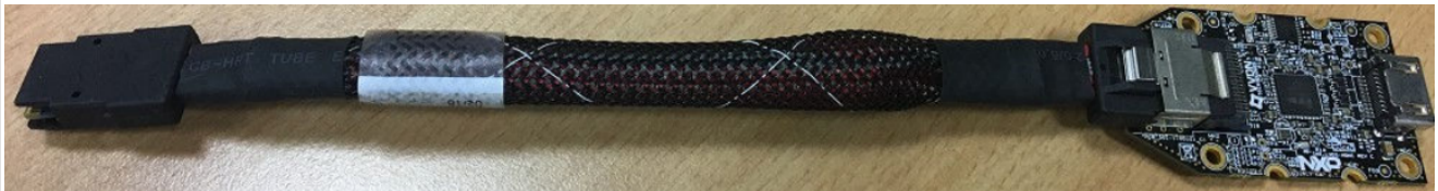
Figure 10. i.MX mini SAS cable with LVDS-to-HDMI adapter
