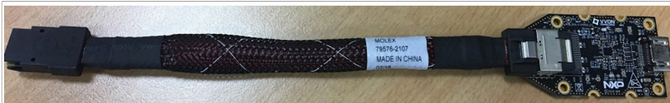
Figure 2. i.MX Mini SAS cable with DSI-to-HDMI adapter IMX-MIPI-HDMI
