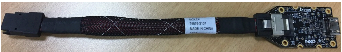
Figure 20. i.MX Mini SAS cable with the DSI-to-HDMI adapter IMX-MIPI-HDMI
