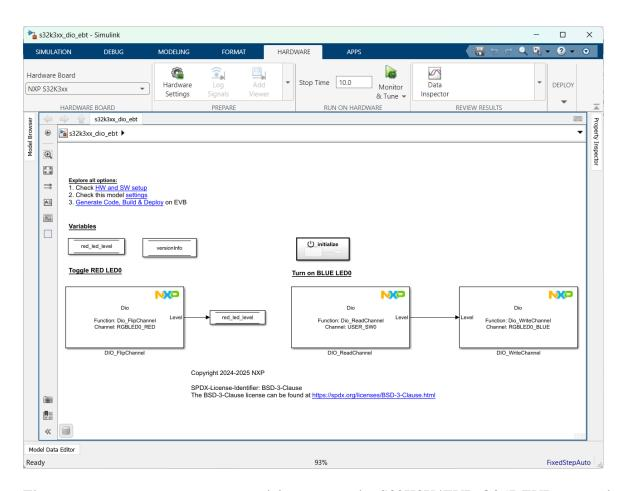
The  $s32k3xx\_dio\_ebt.mdl$  model programs the S32K3X4EVB-Q257 EVB to toggle the D33 red LED every 0.1 seconds. Additionally, if SW4 is pressed, the D32 blue LED should turn on.
