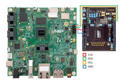
Connect OM-SE051ARD-H to i.MX 8M Mini 8MMINID4-EVK Connect OM-SE051ARD-H to i.MX 8M Nano 8MNANOLPD4-EVK
