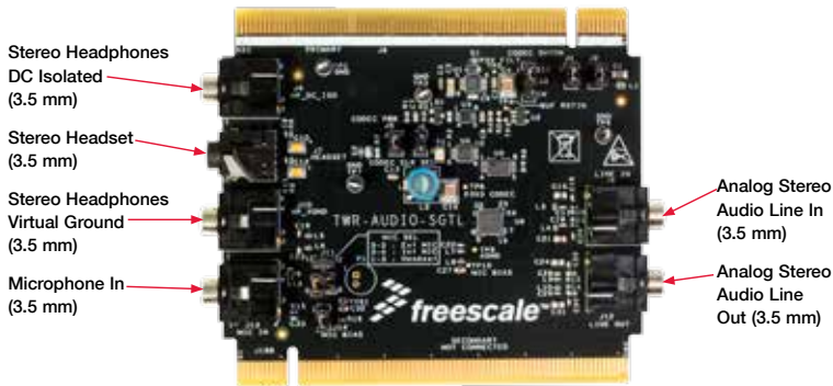
Figure 1: Front Side of TWR-AUDIO-SGTL Module
