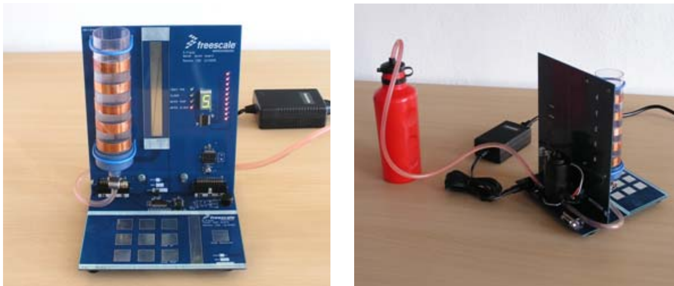
Figure 6-2. E-Field demo (TPB connected with WLB)
