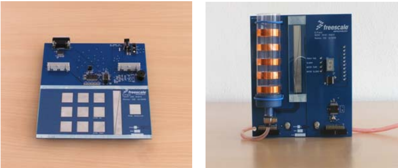
Figure 6-1. E-Field (Touch Pad Board, Water Level Board)
