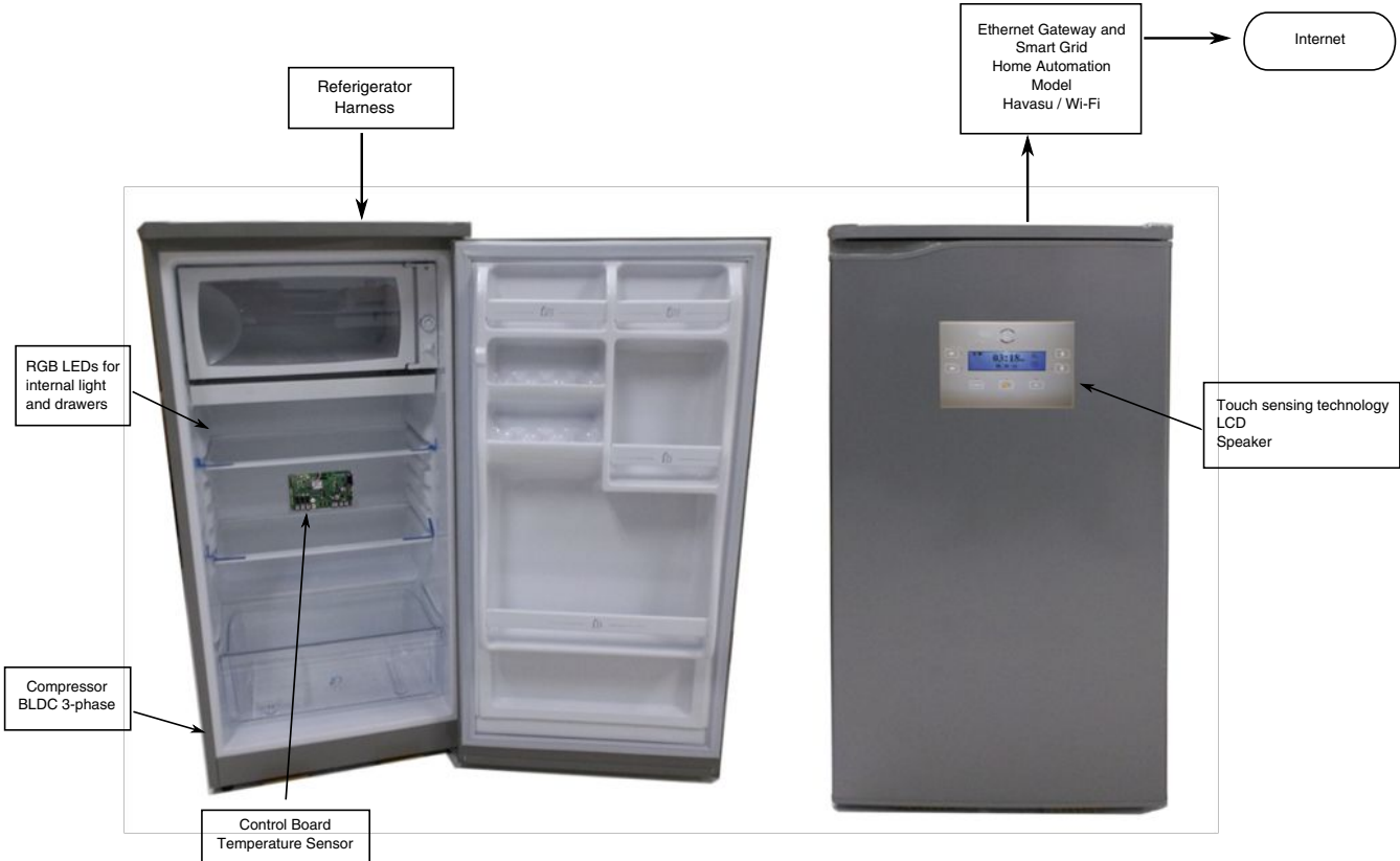
Figure 1-1. Smart appliance sections block diagram
