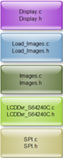
Figure 3-32. High-end display SW modules
