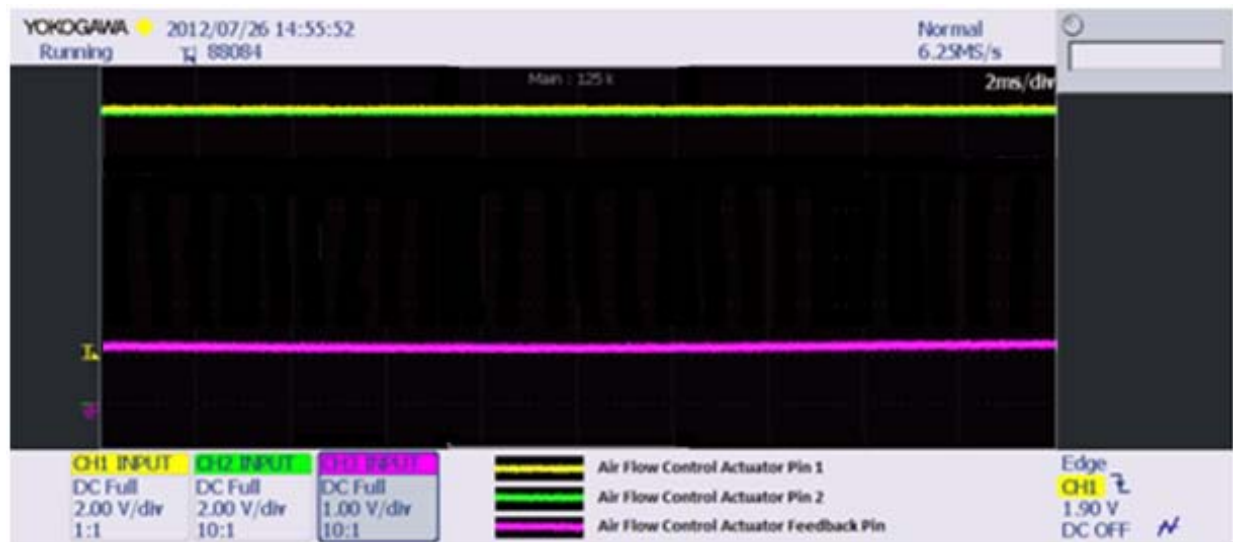
Figure 36. Air flow actuator motor control waveform for defrost position to face & foot position – final phase
