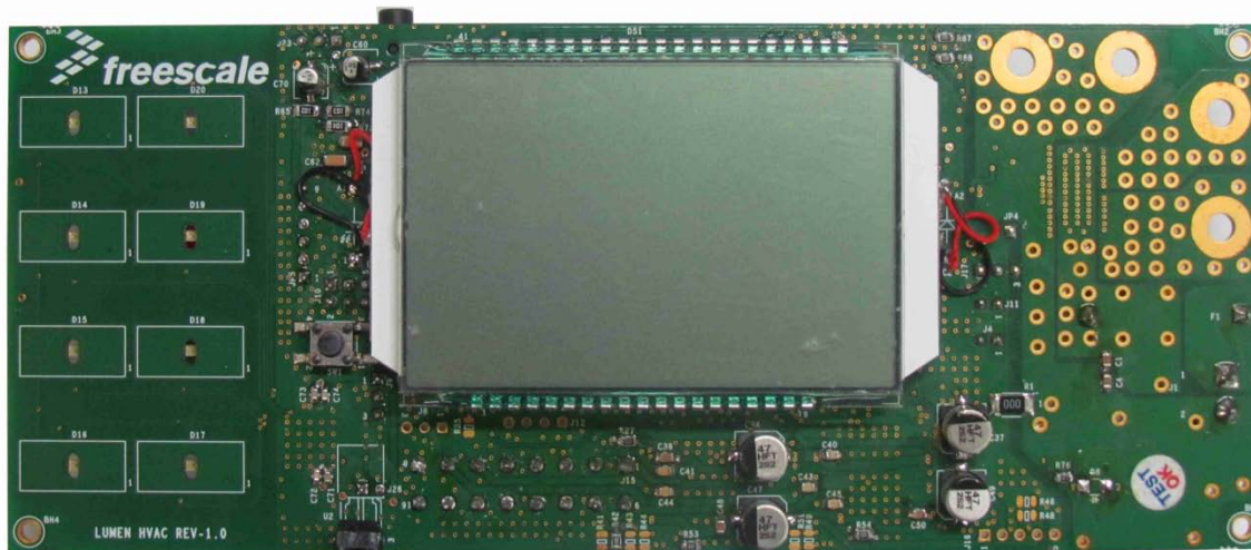
Figure 5. MC9S12ZVH128-based HVAC reference design PCB-LCD side
