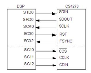
Figure 2-7. Codec Digital Interface Connections
