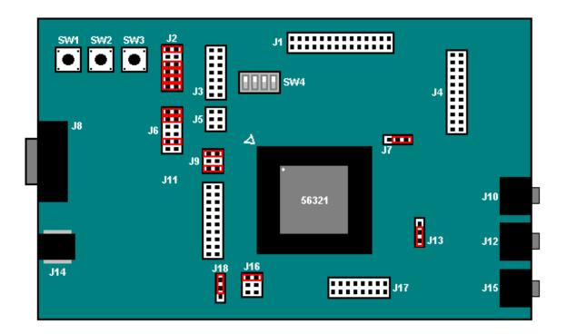
Figure 1-1. DSP563XXEVME Component Layout
