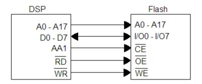
Figure 2-5. Flash Connections
