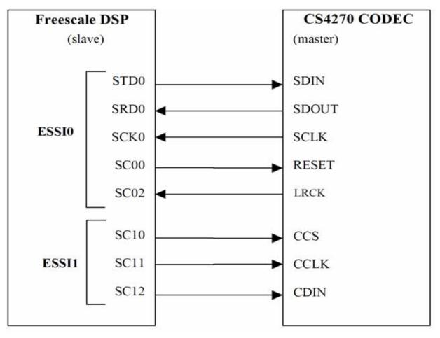
Figure A-2. ESSI/Codec Pin Diagram
