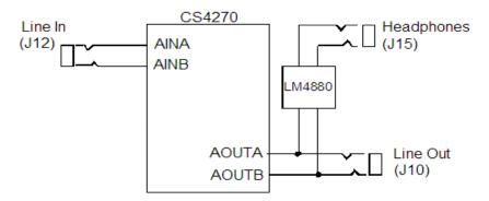
Figure 2-6. Codec Analog Input/Output Diagram
