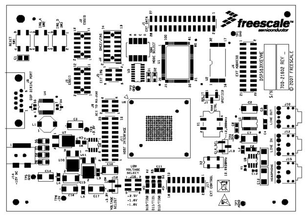
Figure 2-1. DSP563XXEVME Component Layout
