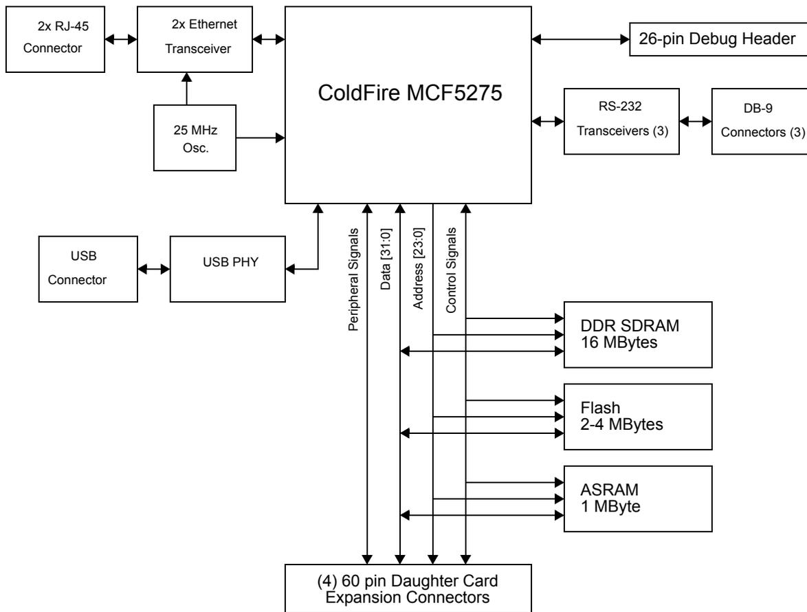
**Figure 1-1. M5275EVB block diagram**
