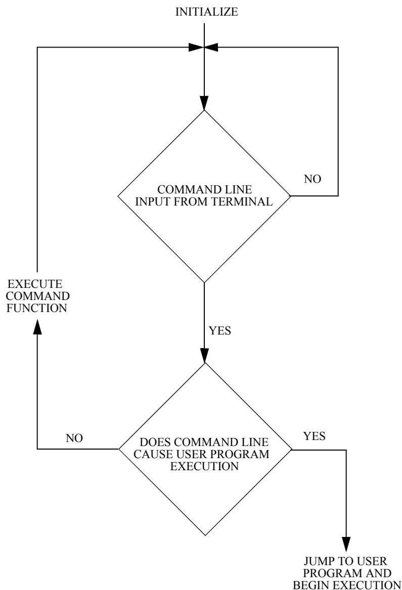
**Figure 3-1. Flow Diagram of dBUG Operational Mode**
