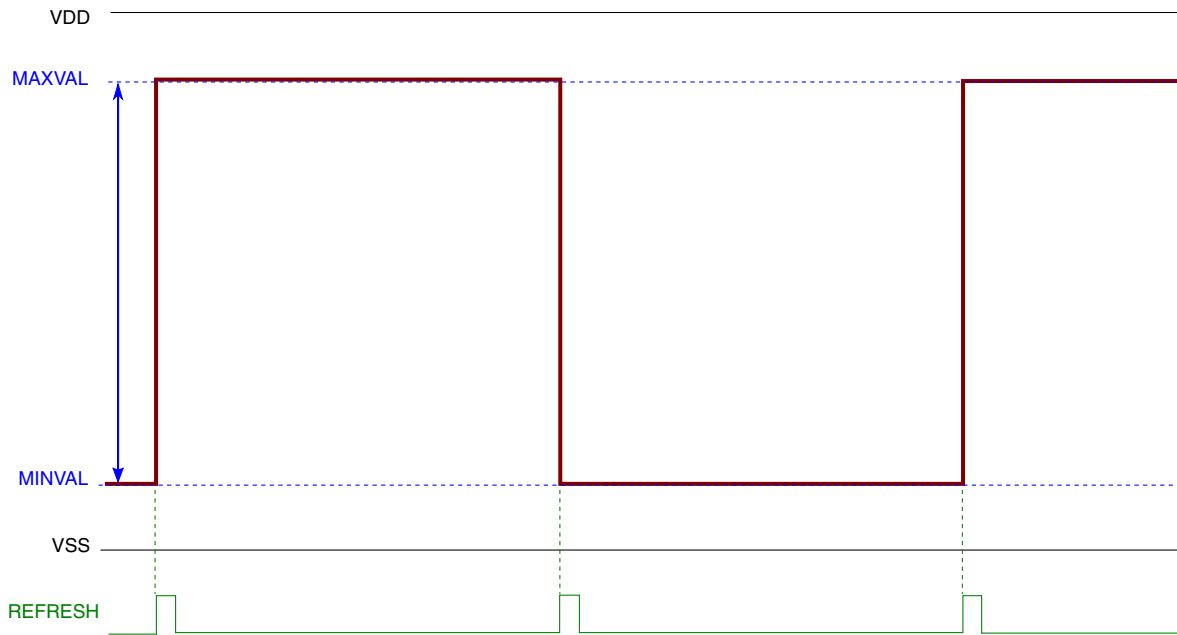
Figure 24-4. Square Waveform Example with CTRL0[UP]=1 and CTRL0[DOWN]=1
