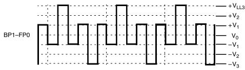
Figure 13-20. "f" Segment Voltage Waveform
