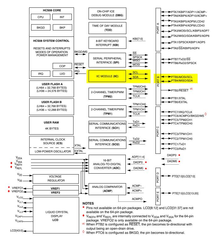
Figure 12-1. MC9S08LH64 Block Diagram Highlighting the IIC Block and Pins
