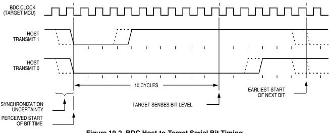
Figure 19-2. BDC Host-to-Target Serial Bit Timing
