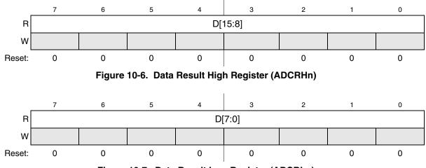
Figure 10-7. Data Result Low Register (ADCRLn)
