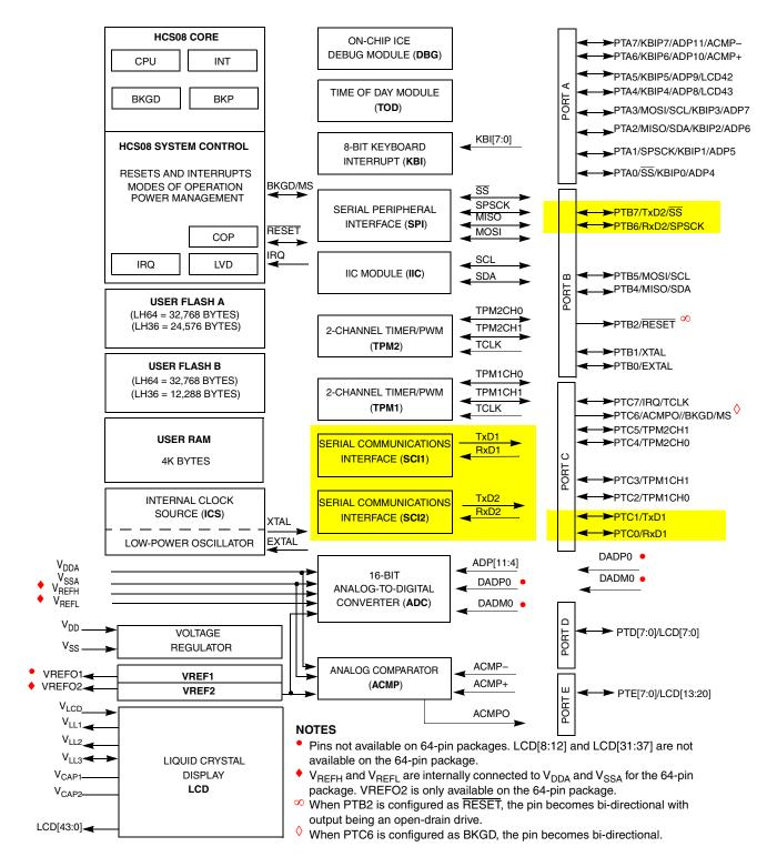
Figure 14-1. MC9S08LH64 Series Block Diagram Highlighting SCI Blocks and Pins
