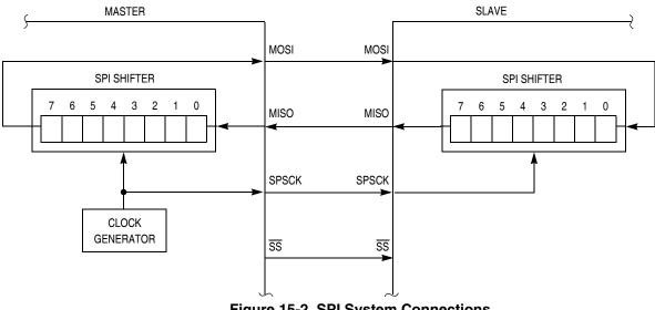
Figure 15-2. SPI System Connections
