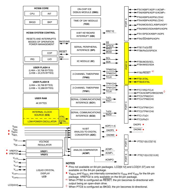
Figure 11-1. MC9S08LH64 Series Block Diagram Highlighting ICS Block and Pins
