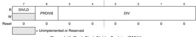
Figure 4-12. Flash Clock Divider Register (FCDIV)
