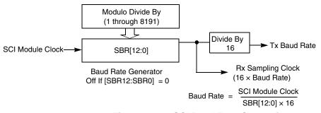
Figure 14-12. SCI Baud Rate Generation
