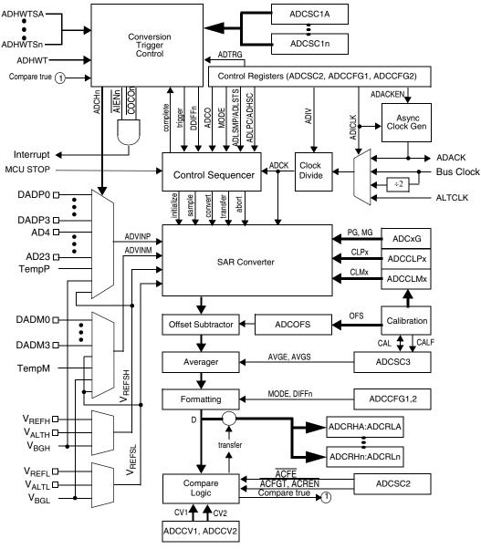
Figure 10-2. ADC Block Diagram
