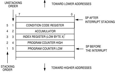
\* High byte (H) of index register is not automatically stacked.
