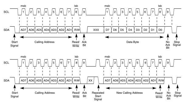
Figure 12-9. IIC Bus Transmission Signals
