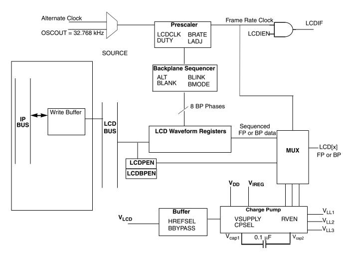
Figure 13-2. LCD Driver Block Diagram
