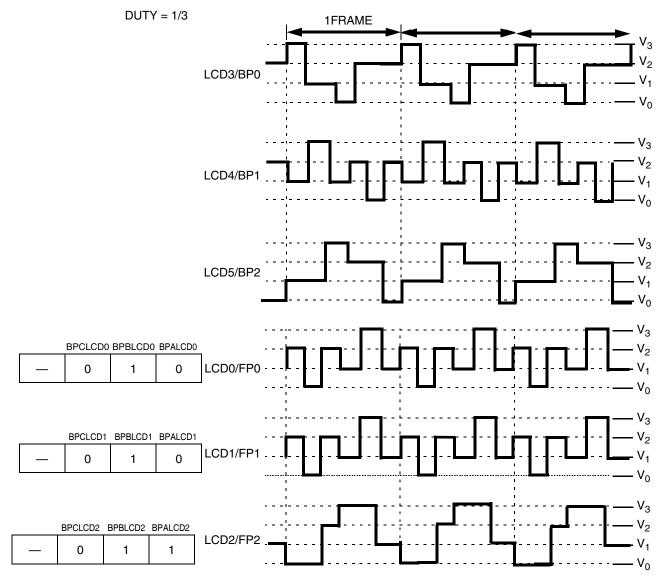
Figure 13-19. LCD Waveforms
