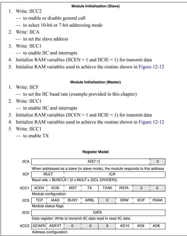
Figure 12-11. IIC Module Quick Start
