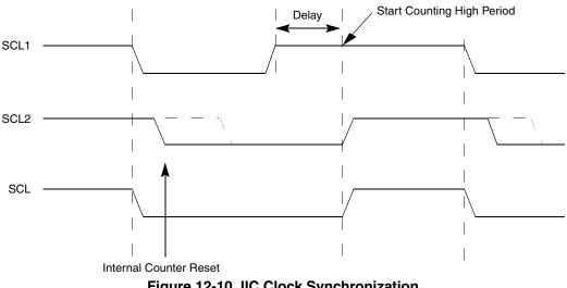
Figure 12-10. IIC Clock Synchronization
