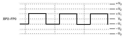
Figure 13-21. "e" Segment Voltage Waveform
