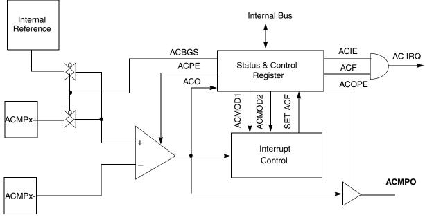
Figure 9-2. Analog Comparator Module Block Diagram
