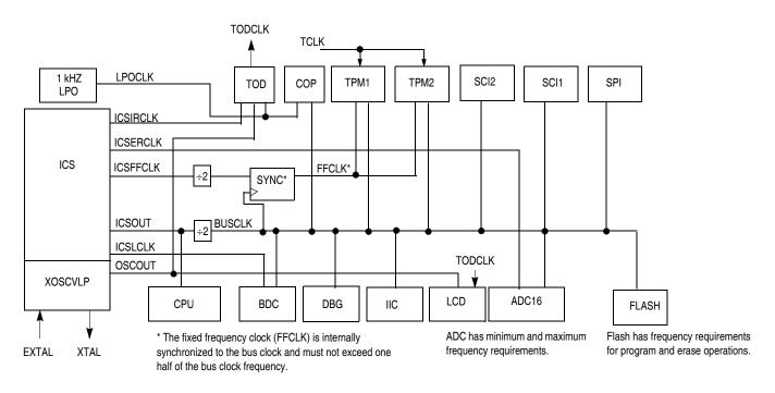
Figure 1-2. System Clock Distribution Diagram
