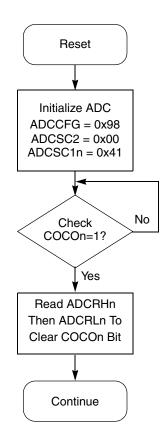
Figure 10-42. Initialization Flowchart for Example
