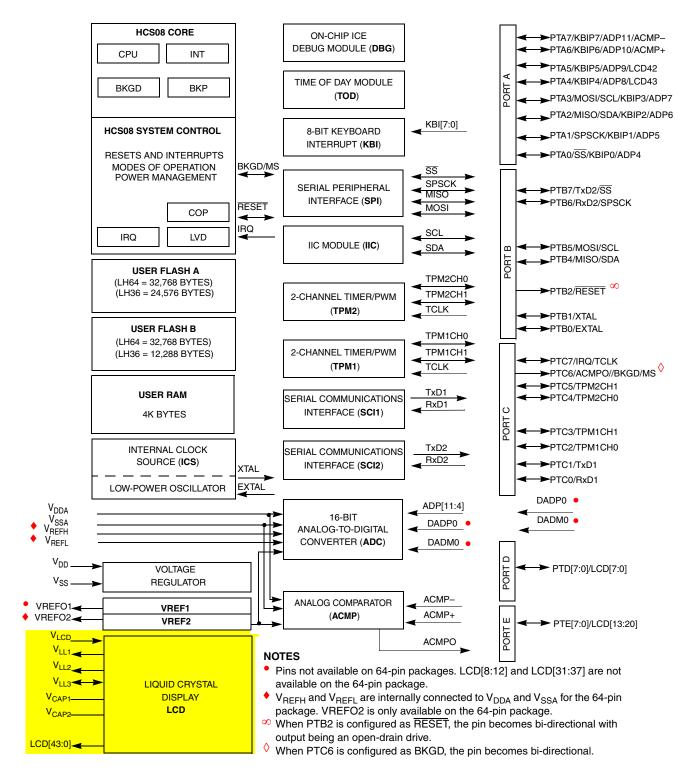
Figure 13-1. MC9S08LH64 Block Diagram Highlighting LCD Block and Pins
