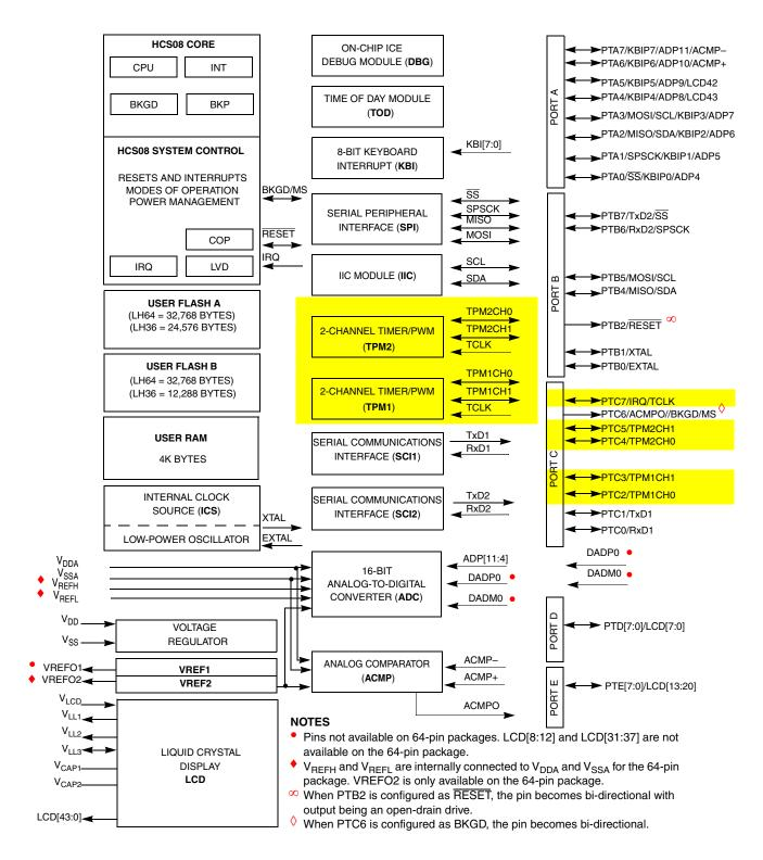
Figure 17-1. MC9S08LH64 Series Block Diagram Highlighting TPM Blocks and Pins
