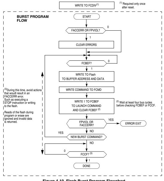
Figure 4-10. Flash Burst Program Flowchart
