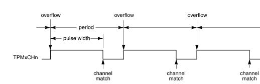
Figure 17-15. EPWM period and pulse width (ELSnA=0)
