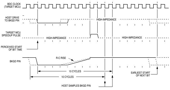
Figure 19-3. BDC Target-to-Host Serial Bit Timing (Logic 1)
