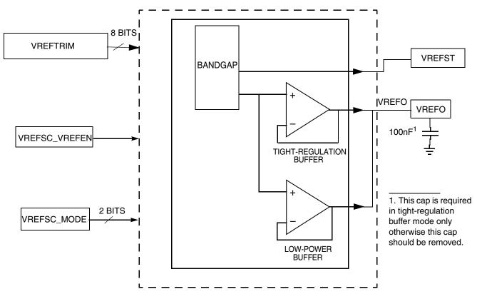
Figure 18-3. Voltage Reference Block Diagram
