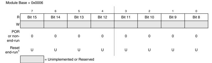
Figure 20-8. Debug FIFO High Register (DBGFH)
