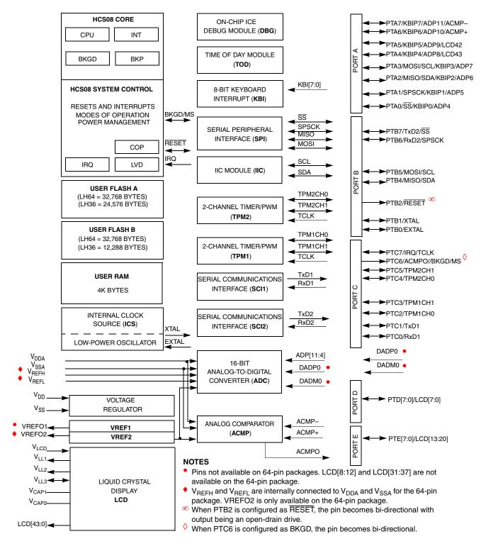
Figure 1-1. MC9S08LH64 Series Block Diagram
