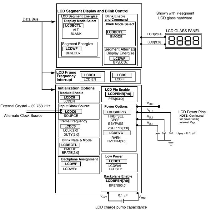
Figure 13-17. LCD Programmer's Model Diagram
