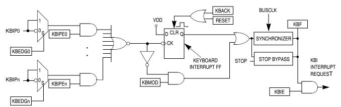
Figure 7-2. Keyboard Interrupt (KBI) Block Diagram
