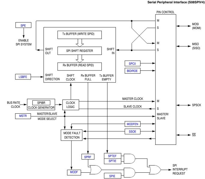
Figure 15-3. SPI Module Block Diagram
