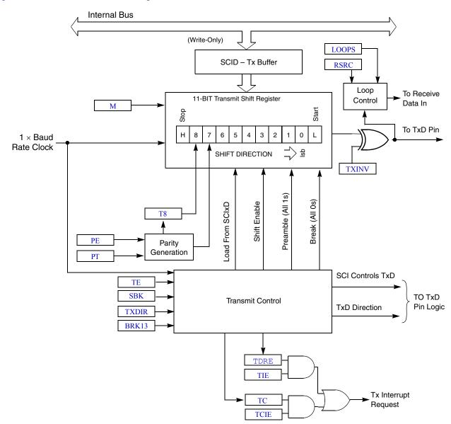
Figure 14-2. SCI Transmitter Block Diagram
