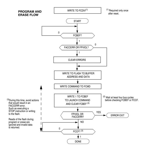
Figure 4-9. Flash Program and Erase Flowchart
