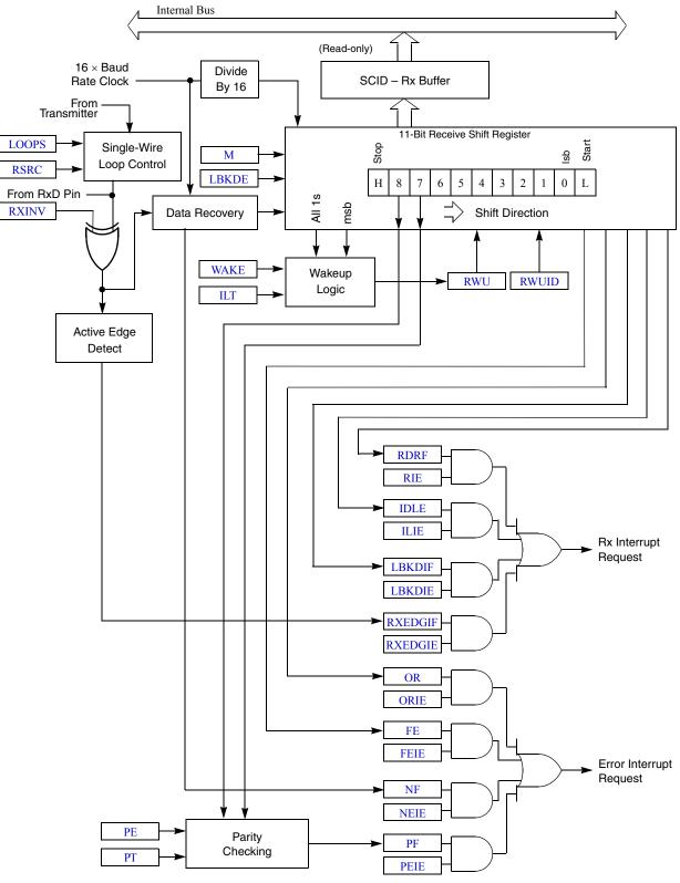
Figure 14-3. SCI Receiver Block Diagram
